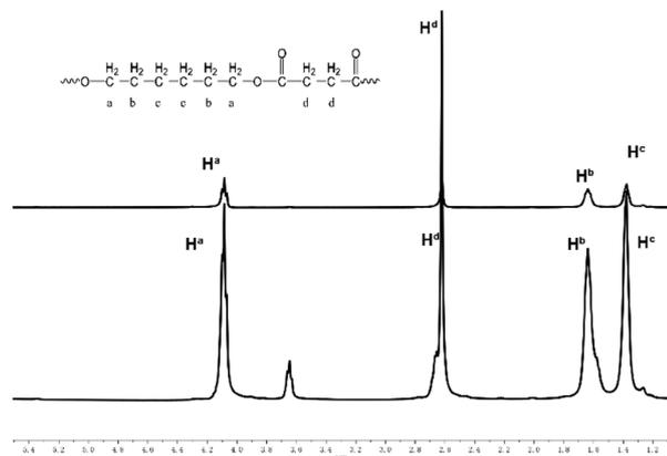
Fig. 3  $^1\text{H}$  NMR spectra ( $\text{CDCl}_3$ , 400 MHz) of oligo(hexylene succinate) at the 2nd hour (below) and poly(hexylene succinate) at the 30th minute (above).
