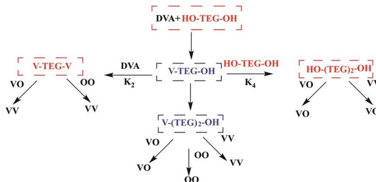
Fig. 8 Scheme of reaction sequences in the transesterification of DVA with TEG.<sup>113</sup>
