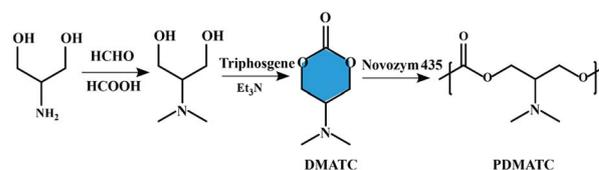
Fig. 3 Schematic representation of the synthesis of six-membered carbonate monomer (DMATC) and water-soluble aliphatic polycarbonate (PDMATC).<sup>42</sup>
