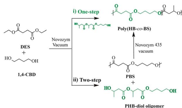
Fig. 5 Schematic of bio-based poly(3-hydroxybutyrate-*co*-butylene succinate) synthesized by enzymatic polycondensation *via* a one-step or two-step Process.<sup>83</sup>
