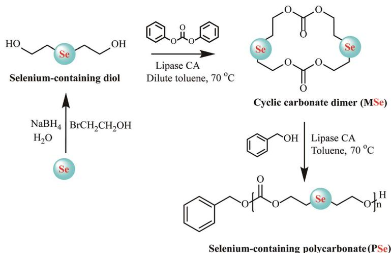
Fig. 4 Schematic representation of selenium-containing polycarbonate (PSe) synthesized by enzymatic ring-opening polymerization.<sup>53</sup>
