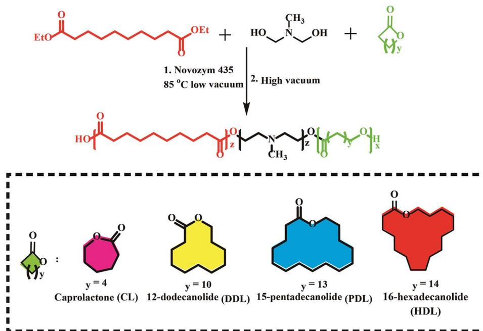
Fig. 6 Schematic of a new biodegradable terpolymerization poly(amine-co-esters) synthesized by a combination of eROP and polycondensation.<sup>95</sup>
