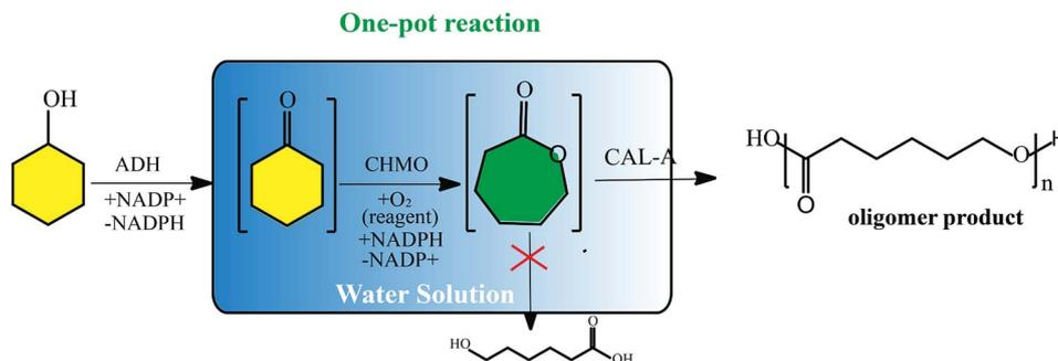
Fig. 2 Schematic representation of the synthesis of the oligomer ( $\epsilon$ -caprolactone) *via* an enzyme cascade.<sup>28</sup>
