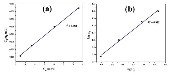
Fig. 11 Adsorption isotherm plots of CV dye (a) Langmuir and (b) Freundlich isotherm.
