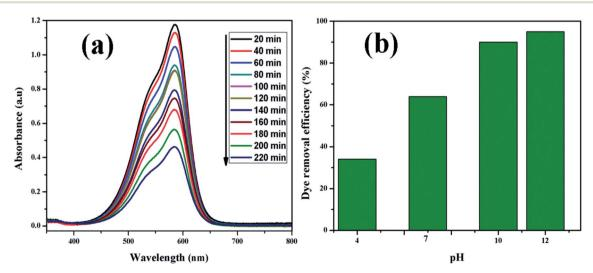
Fig. 9 (a) UV-vis absorption spectrum of CV (20 mg  $L^{-1}$ ) adsorbed on rGO/Fe<sub>3</sub>O<sub>4</sub> NCs at different time and (b) effect of pH on dye removal.
