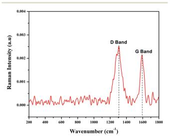
Fig. 4 FT-Raman spectrum of rGO/Fe<sub>3</sub>O<sub>4</sub> NCs.
