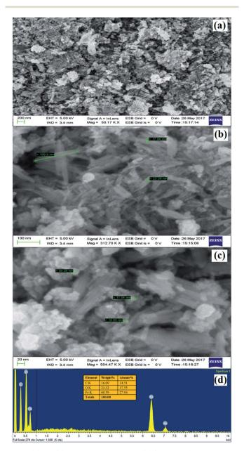
Fig. 6 (a) to (c) FE-SEM images of  $rGO/Fe_3O_4$  NCs at different magnifications and (d) EDX spectrum of  $rGO/Fe_3O_4$  NCs.
