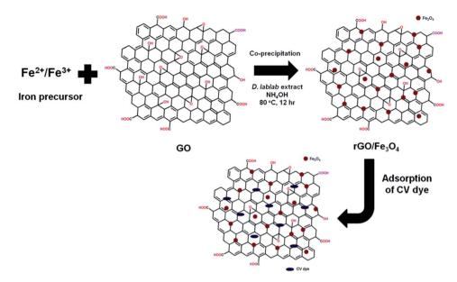
Fig. 1 Proposed mechanism of synthesis of rGO/Fe<sub>3</sub>O<sub>4</sub> NCs using *Dolichos lablab* L. extract and removal of crystal violet dye by adsorption.
