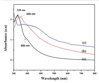
Fig. 2 UV-vis spectra of (a) GO, (b) rGO and (c) rGO/Fe<sub>3</sub>O<sub>4</sub> NCs.
