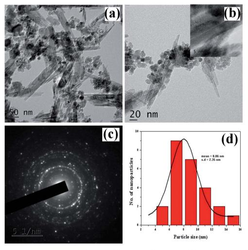
Fig. 7 TEM images of *Dolichos lablab* L. mediated  $rGO/Fe_3O_4$  NCs (a) 50 nm scale, (b) 20 nm scale, (c) SAED patterns of  $rGO/Fe_3O_4$  NCs, and (d) size distribution histogram of  $rGO/Fe_3O_4$  NCs.
