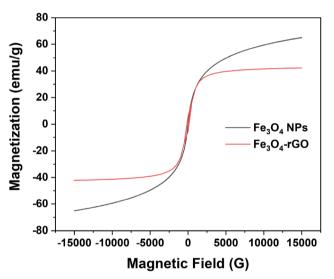
Fig. 8 Room temperature magnetization curve of pure magnetite and rGO/Fe  $_{\tau}O_4$  NCs.
