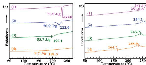
Fig. 2 Differential scanning calorimetry curves in the (a) first cooling and (b) second heating cycles both at a rate of  $10\text{ }^\circ\text{C min}^{-1}$  for (1) non-ionised polyamide (PA)-66, and for PA-66 ionenes bearing (2) 2.3, (3) 6.5 and (4) 11.4 mol% of  $\text{Ca}^{2+}$  ions in their backbone chains which are prepared from solution reactions of PA-66 with  $\text{CaCl}_2$  in formic acid.
