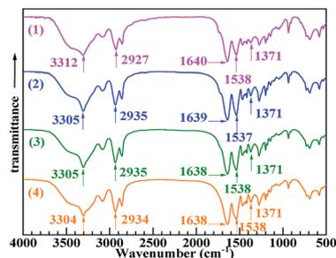
Fig. 1 Fourier transform infrared absorption spectra of (1) non-ionised polyamide (PA)-66, and of PA-66's modified with (2) 2.0, (3) 5.0 and (4) 10.0 wt% of  $\text{CaCl}_2$  (presumably PA-66 ionenes bearing  $\text{Ca}^{2+}$  ions in their backbone chains) which are prepared from solution reactions of PA-66 with  $\text{CaCl}_2$  in formic acid.
