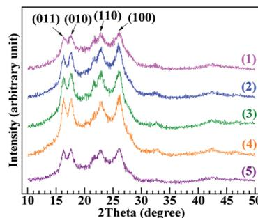
**Fig. 6** Wide-angle X-ray diffractograms of (1) neat poly(ethylene terephthalate) (PET), and of PET matrices nucleated with 5.0 wt% of polyamide (PA)-66 ionenes containing increasing contents of  $\text{Ca}^{2+}$  ions in the backbone chains (mol%): (2) 0 (*i.e.* non-ionised PA-66); (3) 2.3; (4) 6.5; (5) 11.4. The ionenes are prepared from solution reactions of PA-66 with 0, 2.0, 5.0 and 10.0 wt% of  $\text{CaCl}_2$  in formic acid, respectively.
