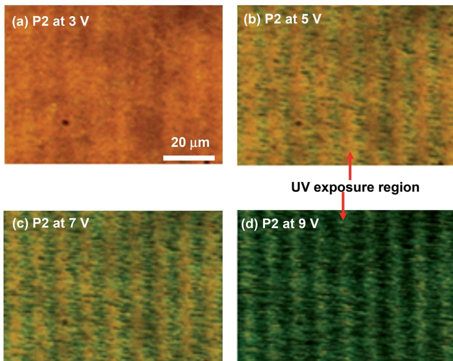
Fig. 7 The microphotographs of the patterned photo-polymerized waveguide LCD P2 under various applied voltages: (a) 0 V, (b) 5 V, (c) 7 V, and (d) 9 V. The scale bar is  $20 \mu\text{m}$ .
