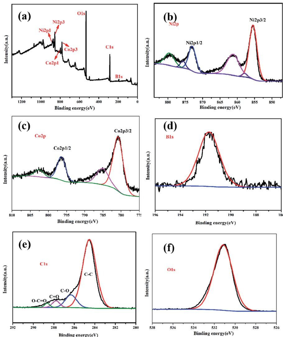
Fig. 6 The full scan XPS spectra of Co1–Ni1–B/RGO/fabric electrode (a); high-resolution XPS spectra of Ni 2p (b), Co 2p (c), B 1s (d) C 1s (e), and O 1s (f).
