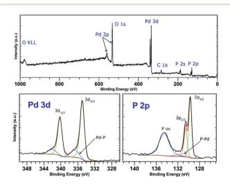
Fig. 4 Survey XPS spectrum (top) and high-resolution spectra of the Pd 4d and P 2p regions (bottom) of Pd-2.
