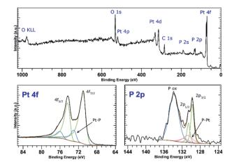
Fig. 6 Survey XPS spectrum (top) and high-resolution spectra of the Pt 4f and P 2p regions (bottom) of Pt-2.
