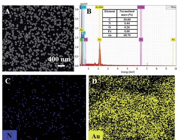
Fig. 6 SEM images (A), EDS (B) and (C and D) elemental mapping images of Au/pDA/Au-PB/CNT/GCE.
