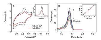
Fig. 7 (A) CVs or DPV (inset) of Ab/Au/pDA/Au-PB/CNT/GCE in absence or presence of CEA (25 ng mL<sup>-1</sup>). (B) DPV curves of Ab/Au/pDA/Au-PB/CNT/GCE towards different concentrations of CEA. (B) The linear relationship between the DPV peak current and the logarithm of concentration of CEA.
