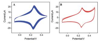
Fig. 4 CVs of (A) Au-PB/CNT/GCE or pDA/Au-PB/CNT/GCE (B) in  $KNO_3$  (0.1 M, pH 7.0) for 20 continuous scans. Scan rate is 50 mV s<sup>-1</sup>.
