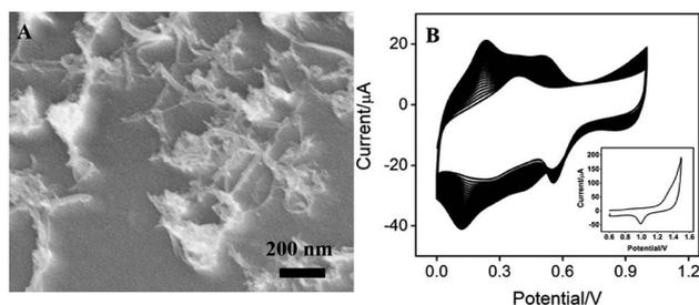
Fig. 1 (A) SEM image of CNT/GCE. (B) CVs of CNT/GCE in KNO<sub>3</sub> solution containing HAuCl<sub>4</sub> and K<sub>3</sub>[Fe(CN)<sub>6</sub>] using consecutive 30 scan cycles (scan rate 50 mV s<sup>-1</sup>). Inset: CV of Au-PB/CNT/GCE in H<sub>2</sub>SO<sub>4</sub> at a scan rate of 100 mV s<sup>-1</sup>.
