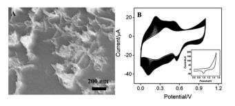
Fig. 1 (A) SEM image of CNT/GCE. (B) CVs of CNT/GCE in  $KNO_3$  solution containing  $HAuCl_4$  and  $K_3[Fe(CN)_6]$  using consecutive 30 scan cycles (scan rate 50 mV s<sup>-1</sup>). Inset: CV of Au-PB/CNT/GCE in  $H_2SO_4$  at a scan rate of 100 mV s<sup>-1</sup>.
