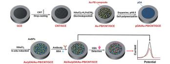
Scheme 1 Schematic illustration for the fabrication of label-free electrochemical immunosensor and reagentless detection of CEA.
