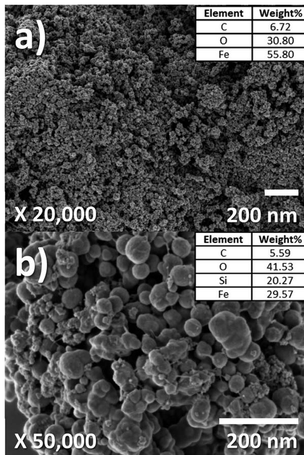
Fig. 3 SEM images and EDX analysis of (a) FeO-NPs and (b) FeO@SiO<sub>2</sub>.
