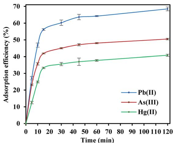
Fig. 7 Adsorption efficiency of the FeO@SiO<sub>2</sub>-DNA for the removal of Pb(II), As(III), and Hg(II).
