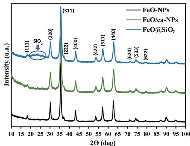
Fig. 4 X-ray diffraction (XRD) patterns showing the characteristic peaks and crystalline nature of the magnetic core and the SiO<sub>2</sub> shell.
