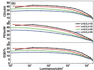
Fig. 7 The EL performance of structured non-doped WOLED with different-thickness exciplex layers. (a) Current density-voltage-luminance curves. (b) CE, PE and EQE-luminance curves.
