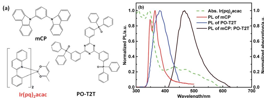
Fig. 1 (a) The molecular structure of **mCP**, **PO-T2T** and **Ir(pq)<sub>2</sub>acac**. (b) The absorption spectrum of **Ir(pq)<sub>2</sub>acac**, and PL spectra of **mCP**, **PO-T2T** and **mCP:PO-T2T** mixed film.
