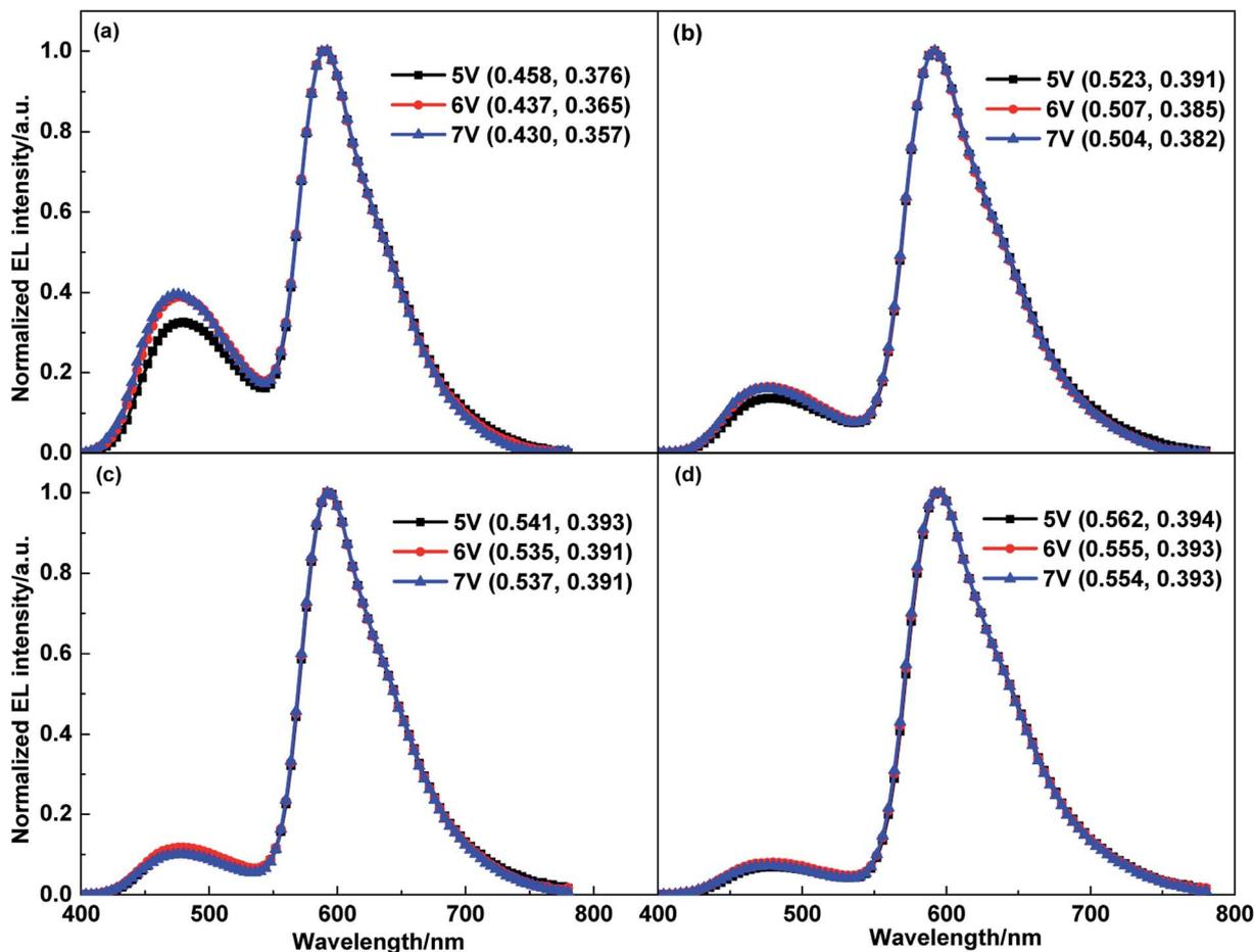
Fig. 5 The EL spectra of structured non-doped WOLED with different ultrathin layer thickness. (a)  $x = 0.2$ . (b)  $x = 0.4$ . (c)  $x = 0.8$ . (d)  $x = 1.1$ .
