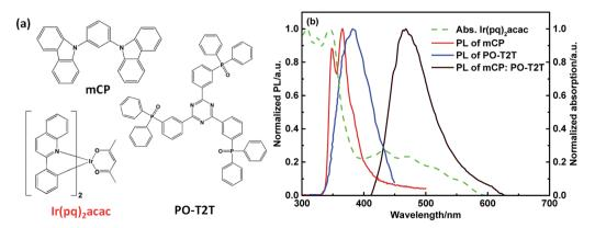
Fig. 1 (a) The molecular structure of mCP, PO-T2T and Ir(pq)₂acac. (b) The absorption spectrum of Ir(pq)₂acac, and PL spectra of mCP, PO-T2T and mCP:PO-T2T mixed film.
