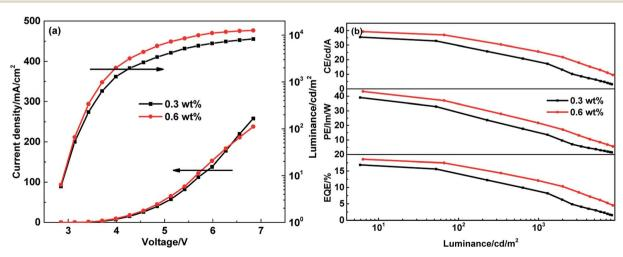
Fig. 2 The EL performance of doped structural WOLED. (a) Current density-voltage-luminance curves. (b) CE, PE and EQE-luminance curves.
