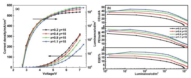
Fig. 4 The EL performance of non-doped structural WOLED with different-thickness ultrathin layers. (a) Current density-voltage-luminance curves. (b) CE, PE and EQE-luminance curves.
