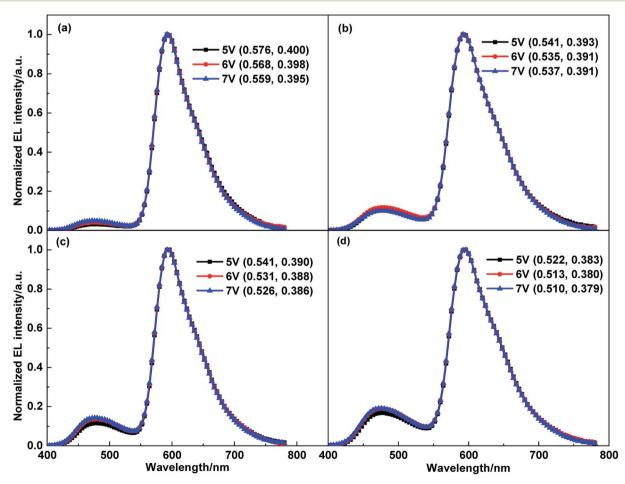
The EL spectra of structured non-doped WOLED with different-thickness exciplex layers. (a) y = 10. (b) y = 15. (c) y = 20. (d) y = 25.
