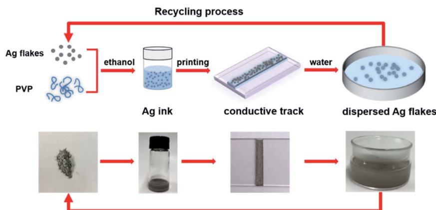
Fig. 1 Schematic illustration of the experimental process of the Ag conductive track.
