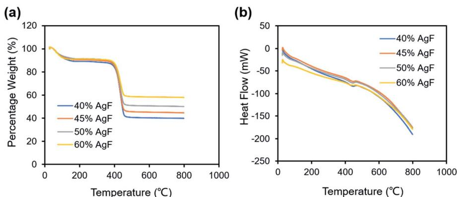
Fig. 3 TGA/DSC result of the AgF/PVP composite.
