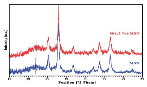
Fig. 3 XRD patterns of the as-synthesized N(1.3 wt%)-MSN and MSN.
