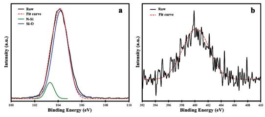
Fig. 5 XPS analysis for N(1.3 wt%)-MSN: (a) deconvolution of the Si 2p, (b) spectrum of N 1s.
