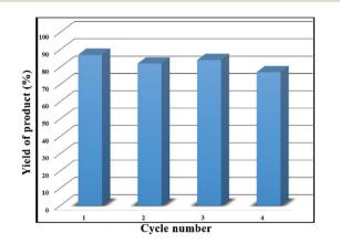
Fig. 6 Reusability of the N(1.3 wt%)-MSN catalyst in the multicomponent reaction.
