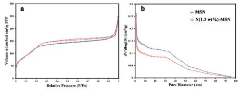
Fig. 4 (a) Nitrogen adsorption-desorption isotherms of MSN and N(1.3 wt%)-MSN, (b) BJH plots of MSN and N(1.3 wt%)-MSN.
