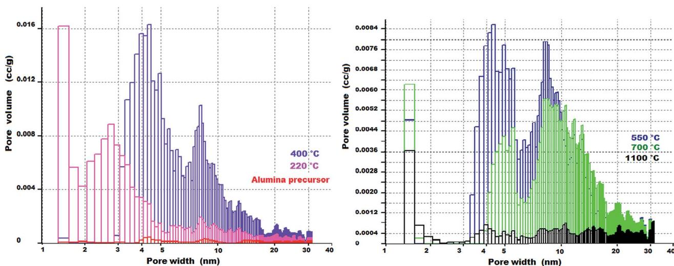
Fig. 9 Pore volume histograms of the prepared alumina precursor and its calcined products obtained at different temperatures determined by DFT.
