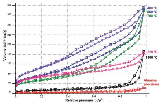
**Fig. 7** N<sub>2</sub> adsorption–desorption isotherms of the prepared alumina precursor and its calcined products obtained at different temperatures.
