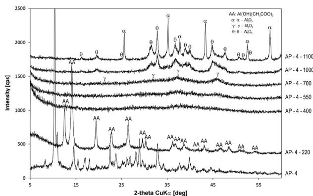
Fig. 4 XRD patterns of the prepared alumina precursor (AP-4) and its thermal decomposition products after calcination at different temperatures for 2 h. Abbreviations: AA:  $\text{Al(OH)(CH}_3\text{COO)}_2$  (ICDD 00-013-0833);  $\alpha$ :  $\alpha\text{-Al}_2\text{O}_3$  (ICDD 01-089-3072);  $\gamma$ :  $\gamma\text{-Al}_2\text{O}_3$  (ICDD 00-010-0425);  $\theta$ :  $\theta\text{-Al}_2\text{O}_3$  (ICDD 01-035-0121).
