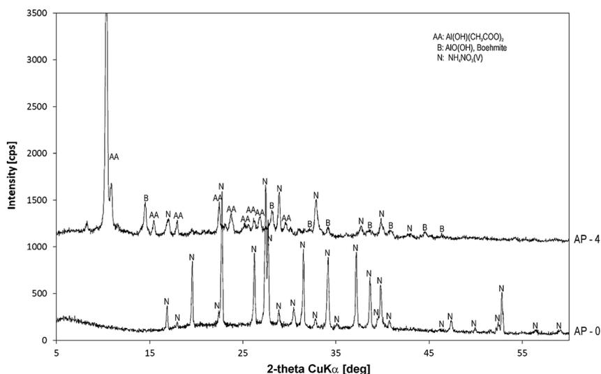
Fig. 2 XRD patterns of the prepared alumina precursor with 4 g Al(OH)(CH<sub>3</sub>COO)<sub>2</sub> (AP-4) and without addition of Al(OH)(CH<sub>3</sub>COO)<sub>2</sub> (AP-0). Abbreviations: AA: Al(OH)(CH<sub>3</sub>COO)<sub>2</sub> (ICDD 00-004-0113); B: boehmite AlO(OH) (ICDD 01-083-1506); N: NH<sub>4</sub>NO<sub>3</sub> (AP-0, ICDD 00-008-0499 and ICDD 01-083-0520; AP-4, ICDD 01-083-0520).
