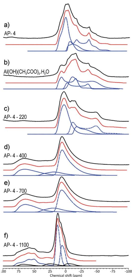
Fig. 6  $^{27}\text{Al}$  NMR spectra of the (a) prepared  $\text{Al}_2\text{O}_3$  precursor (AP-4), (b)  $\text{Al}(\text{OH})(\text{CH}_3\text{COO})_2 \cdot \text{H}_2\text{O}$ , and the prepared  $\text{Al}_2\text{O}_3$  precursor calcined at (c) 220, (d) 400, (e) 700, and (f) 1100 °C (black: experimental; color: simulated).
