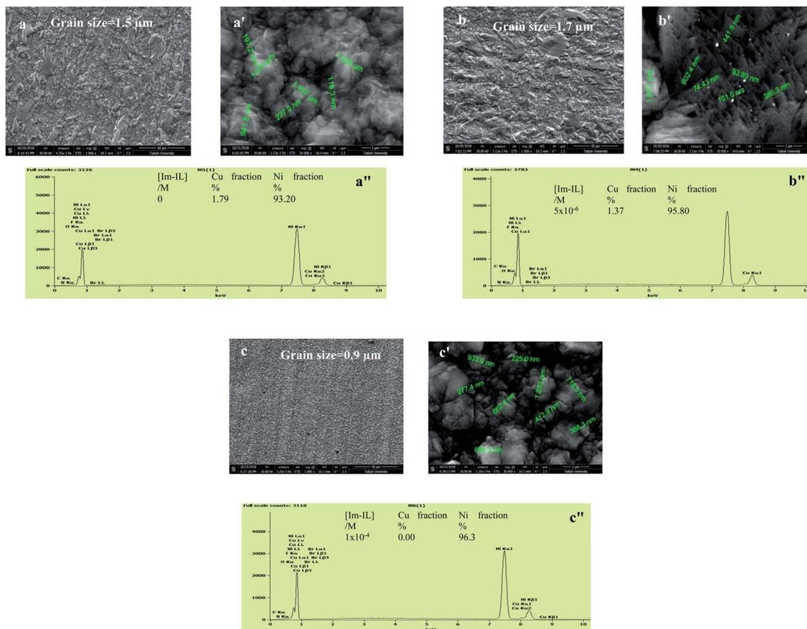
Fig. 6 SEM images, high magnification SEM and EDX spectra of Ni deposited from bath (a, a' and a'') free Im-IL, (b, b' and b'')  $1 \times 10^{-4}$  M Im-IL, (c, c' and c'')  $5 \times 10^{-6}$  M Im-IL.
