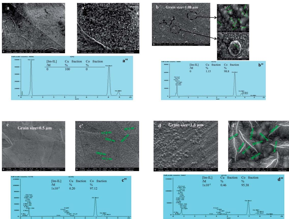
Fig. 5 SEM images, high magnification SEM and EDX spectra of (a, a' and a'') Cu substrate, Co deposited from bath (b, b' and b'') free Im-IL, (c, c' and c'')  $1 \times 10^{-5} \text{ M}$  Im-IL, (d, d' and d'')  $1 \times 10^{-3} \text{ M}$  Im-IL.
