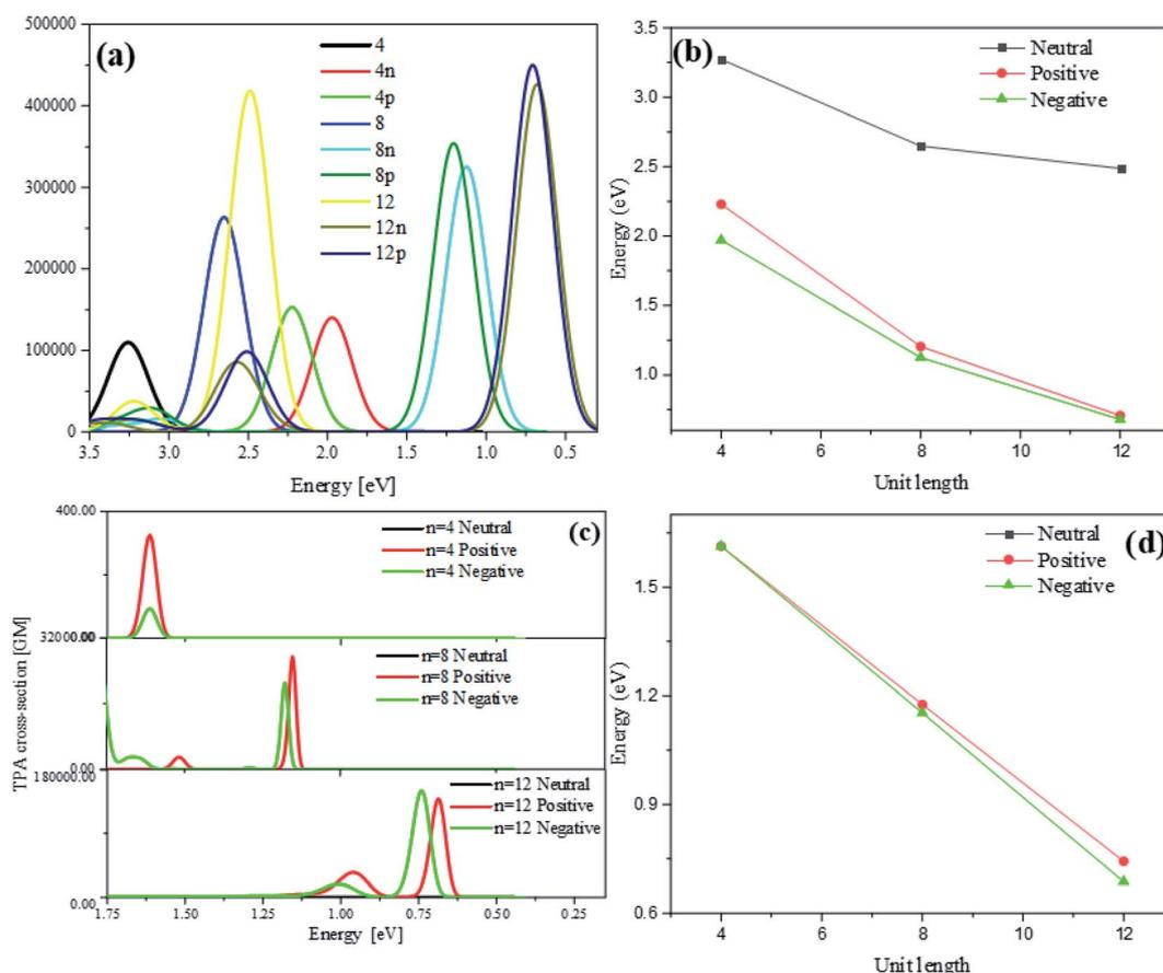
Fig. 3 The OPA (a) and TPA (c) spectra of different length thiophene oligomer. The change of excitation energy of neutral, positive and negative system strongest absorption peaks in  $S_1$  of OPA (b) and  $S_2$  of TPA (d).
