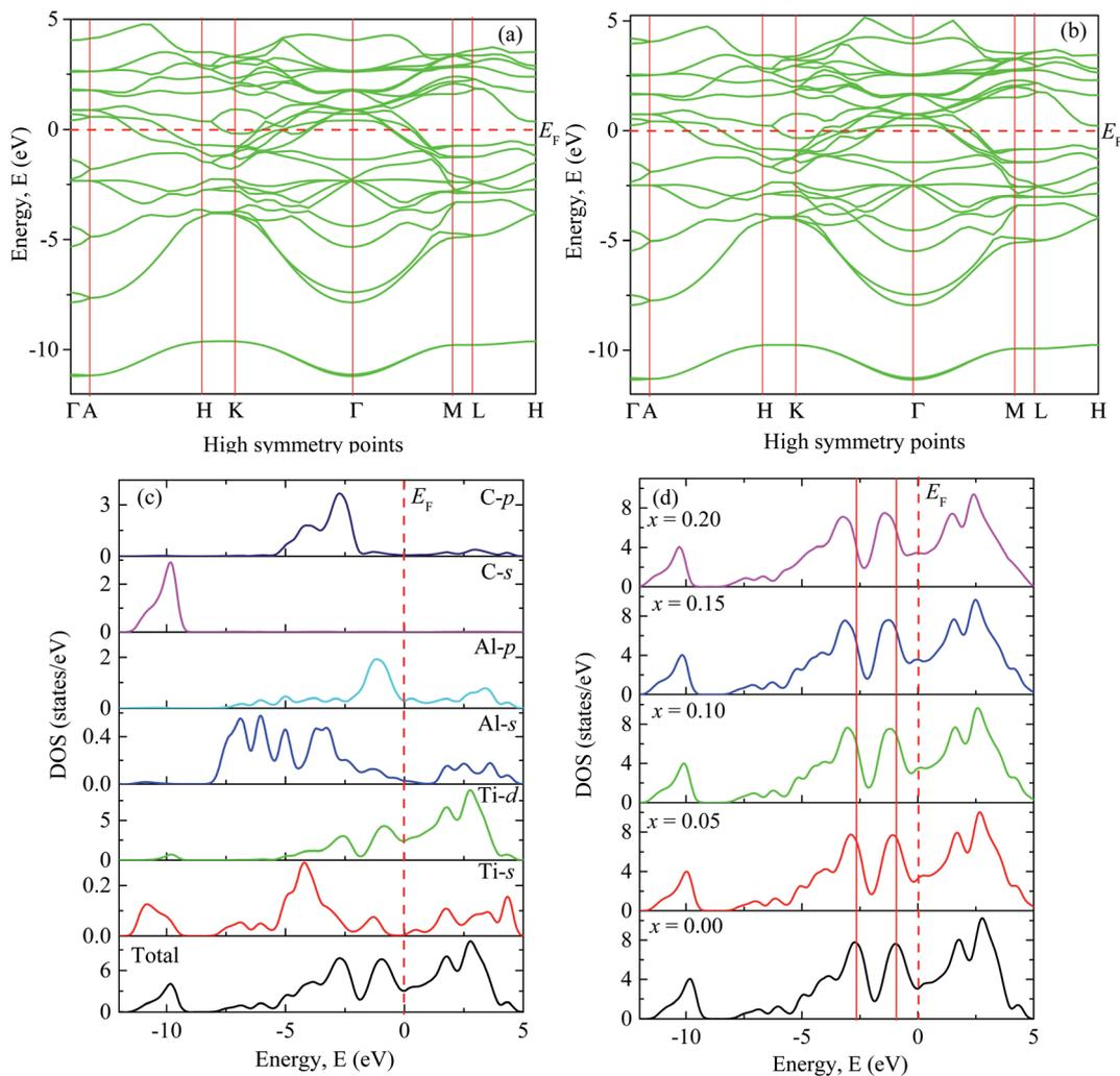
Fig. 2 The electronic band structure of (a)  $\text{Ti}_2\text{AlC}$  and (b)  $(\text{Ti}_{0.95}\text{Mo}_{0.05})_2\text{AlC}$ . Total and partial DOS of (c)  $\text{Ti}_2\text{AlC}$  and (d) the total DOS for different Mo contents.
