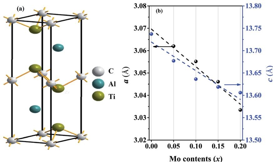
Fig. 1 (a) Crystal structure (unit cell) of the  $\text{Ti}_2\text{AlC}$  compound and (b) lattice constants  $a$  (Å) and  $c$  (Å) for different Mo contents (the linear fits to the lattice constants are also shown).
