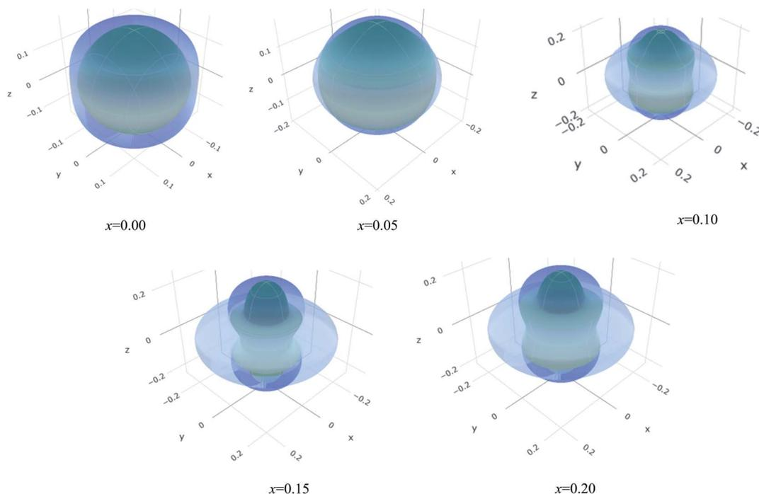
Fig. 8 The three-dimensional contour plots of the Poisson's ratio for  $(\text{Ti}_{1-x}\text{Mo}_x)_2\text{AlC}$  solid solutions.
