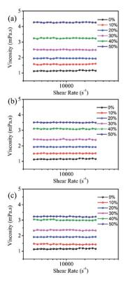
Fig. 6 The rheological property of 100 mM Orange 13 dye aqueous solution containing different organic solvents at 25 °C. (a) EG, (b) MOE and (c) DME
