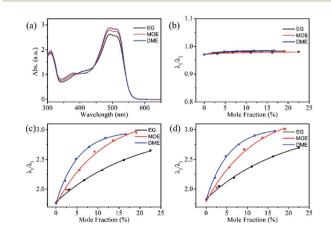
Fig. 3 (a) UV-vis absorption spectra of dye solution containing 100 mM Orange 13 and 30% organic solvent. The ratio of the different absorption peak intensity of the UV-vis absorption spectrum, (b)  $\lambda_1/\lambda_2$ , (c)  $\lambda_1/\lambda_3$ , (d)  $\lambda_2/\lambda_3$ .
