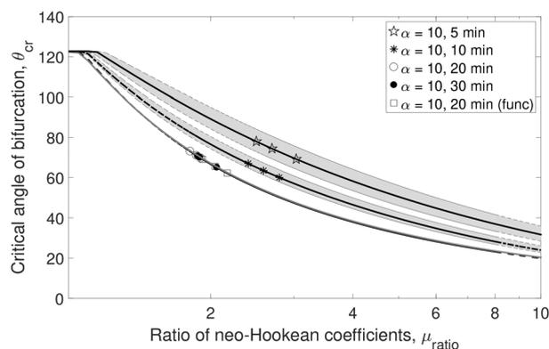
**Fig. 3** The methodology introduced in Sinha *et al.*, 2019,<sup>17</sup> employed to estimate neo-Hookean coefficient for SiNC layers corresponding to parametric variation. The lines represent the numerical solution for the average of thickness ratios ( $t$ ) for a given sample deposition time, and the symbols represent experimental data points. The shaded region shows an area of one standard deviation of the thickness ratio from average for the samples.
