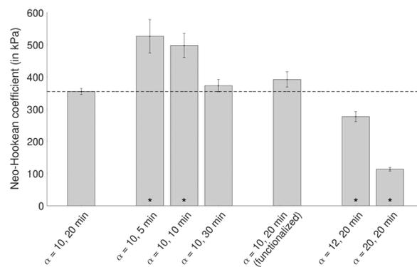
**Fig. 2** Neo-Hookean coefficient of all samples. The samples with asterisks indicate sample conditions that led to neo-Hookean coefficients that deviated with statistical significance from samples reported in ref. 17 ( $\alpha = 10$ ,  $t = 460$ ).
