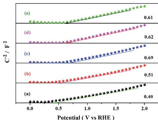
Fig. 10 Mott-Schottky diagram of the catalyst at 500 Hz in 0.2 M  $\text{Na}_2\text{SO}_4$  solution.
