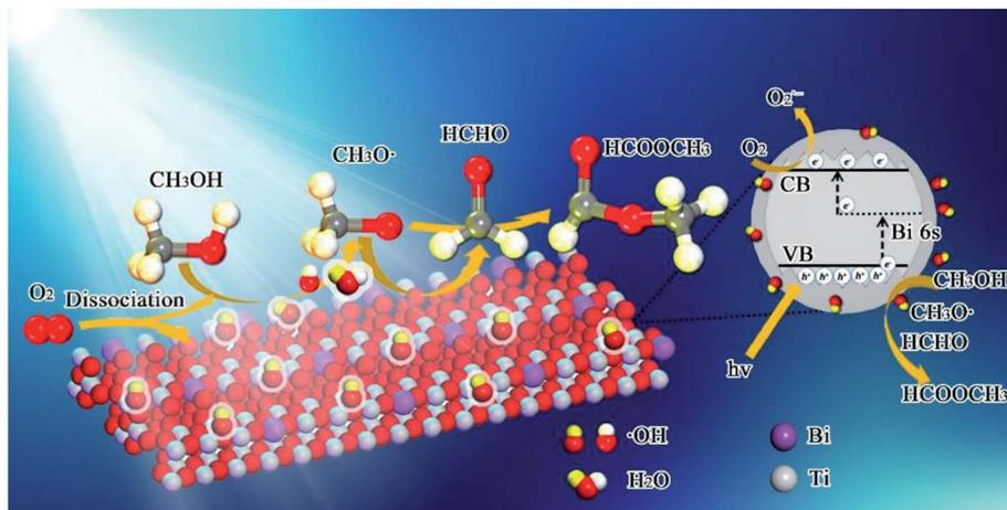
Fig. 14 Reaction mechanism of selective oxidation of methanol to methyl formate with Bi-TiO<sub>2</sub> catalyst under simulated sunlight.
