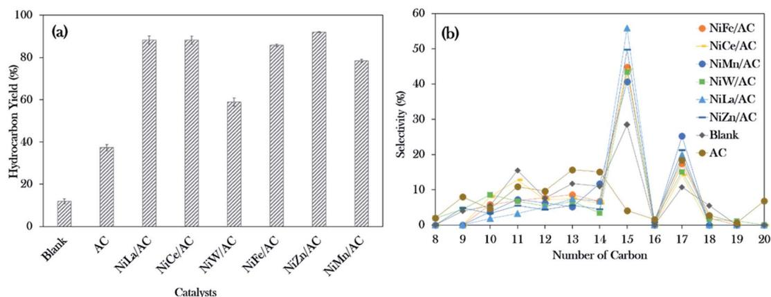
Fig. 5 Data collected from the deoxygenation process: (a) hydrocarbon yield and (b) *n*-(C<sub>15</sub> + C<sub>17</sub>) selectivity for blank and catalysed deoxygenation (operating parameters: 3 wt% of catalyst loading, 350 °C reaction temperature, 2 h reaction time under inert conditions).
