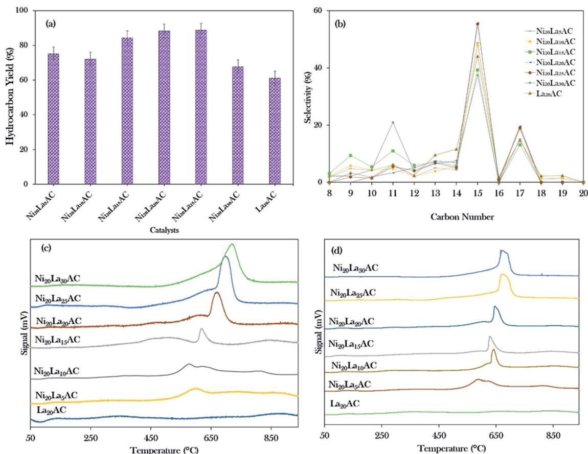
Fig. 8 (a) Hydrocarbon yield, (b) hydrocarbon selectivity, (c) TPD-NH<sub>3</sub>, (d) TPD-CO<sub>2</sub> for the catalytic deoxygenation of WCO over different concentrations of La (5–30 wt%).
