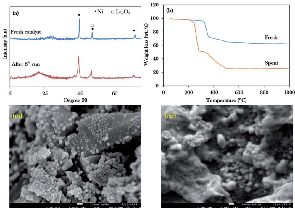
Fig. 11 Stability studies of the Ni<sub>20</sub>La<sub>20</sub>AC catalyst for the 6<sup>th</sup> run: (a) the XRD profile, (b) TGA, (ci) FESEM image for the fresh catalyst, (cii) FESEM image for the spent catalyst.
