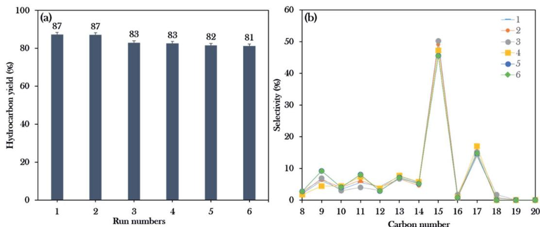
Fig. 10 Reusability studies of the Ni<sub>20</sub>La<sub>20</sub>AC catalyst for the 6<sup>th</sup> run: (a) the hydrocarbon yield profile, (b) hydrocarbon selectivity.
