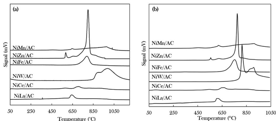
**Fig. 3** Temperature-programmed desorption patterns of (a) TPD-NH<sub>3</sub> and (b) TPD-CO<sub>2</sub> of binary metal oxide-supported AC catalysts.
