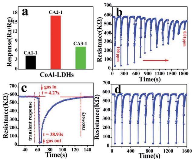
Fig. 7 Gas sensitivity of (a) different ratio CoAl-LDHs samples to 100 ppm  $\text{NO}_x$ , (b) CA2-1 to 100–0.01 ppm  $\text{NO}_x$ , (c) response–recovery to 100 ppm  $\text{NO}_x$  and (d) CA2-1 response to 100 ppm  $\text{NO}_x$ .
