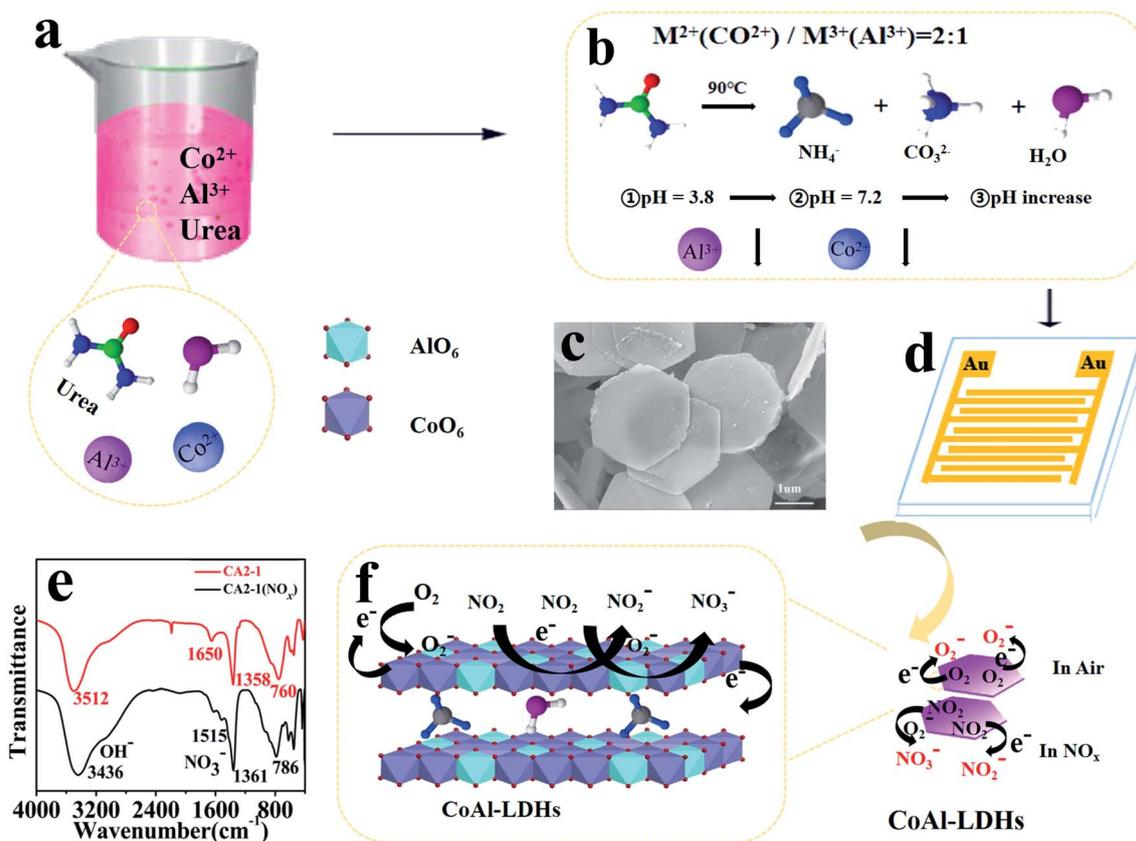
Scheme 1 The formation and gas-sensing mechanism of the 2D nanosheet structure of  $\text{CoAl-LDHs}$ . (a) Reaction beaker, (b) process of reaction, (c) two-dimensional (2D) nanosheet structure of CA2-1, (d) Au electrode, (e) FT-IR spectra of CA2-1 before and after adsorption of  $\text{NO}_x$  (test for 2 h), and (f) LDH assembly structure.
