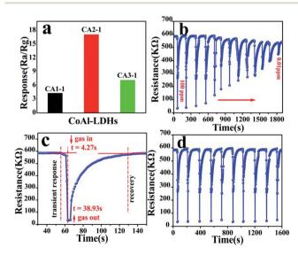
Fig. 7 Gas sensitivity of (a) different ratio CoAl-LDHs samples to  $100 \text{ ppm NO}_x$ , (b) CA2-1 to  $100-0.01 \text{ ppm NO}_x$ , (c) response-recovery to  $100 \text{ ppm NO}_x$  and (d) CA2-1 response to  $100 \text{ ppm NO}_x$ .
