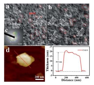
Fig. 5 (a and b) HRTEM images, (c) selected-area electron diffraction (SAED) pattern and (d) AFM images and height profiles of the CA2-1 sample.
