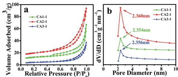
Fig. 2 BET of CA1-1, CA2-1 and CA3-1 samples: (a) specific surface area, and (b) pore diameter distribution curves.
