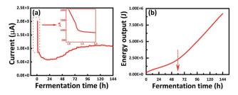
Fig. 4 Electricity generation performance during the incubation. (a) Current monitoring with 2  $\Omega$  resistor; (b) cumulative energy output in the whole BC fermentative production.
