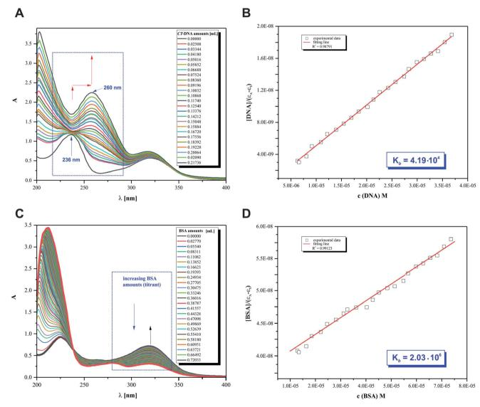
Fig. 10 Absorption spectra of 2HP in Tris–HCl buffer upon the addition of (A) CT-DNA (0.37 mM) with subtraction of the CT-DNA absorbance ([2HP] = 0.18 mM). (B) Plot of [DNA]/( $\varepsilon_a - \varepsilon_f$ ) vs. [DNA]. (C) BSA (0.25 mM) with subtraction of the BSA absorbance ([2HP] = 0.12 mM). (D) Plot of [BSA]/( $\varepsilon_a - \varepsilon_f$ ) vs. [BSA]. The arrows show the absorbance changes associated with an increase in biomolecule concentration.
