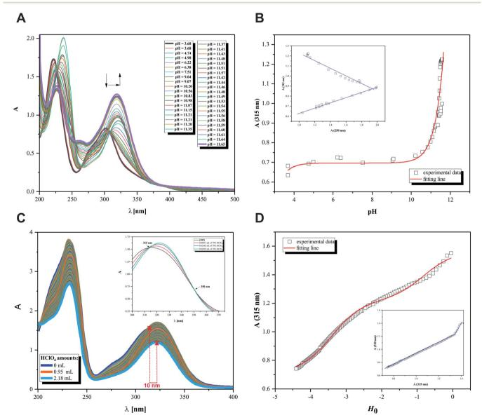
Fig. 7 Spectrophotometric results. (A) UV spectral curves of 2HP (0.18 mM) as a function of pH (3.68-11.65). (B) Absorption at 315 nm vs. measured pH, where experimental data presented as squares and calculation results shown as red line;  $R^2 = 0.98721$ . (C) Titration curves from Hammett's acidity function. (D) Absorption at 315 nm vs. Ho index, where experimental data presented as squares and calculation results as red line;  $R^2 = 0.99647$ .
