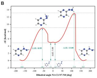
Fig. 4 Energy variation curve of the dihedral angle of N1–C2–N7–N8 in 2-hydrazinopyrazine during the transition of the conformers. (A) 2HP(A) into 2HP(C) and (B) 2HP(B) into 2HP(D).
