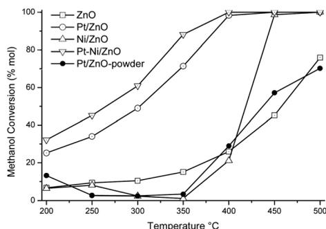
Fig. 5 Temperature dependence of ARM activity of catalysts.
