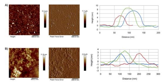
Fig. 3 AFM results for (A) CNO-CDs and (B) GO-CDs, showing, from left to right, topography, peak force error and height profile along with the lines evidenced in topography images.
