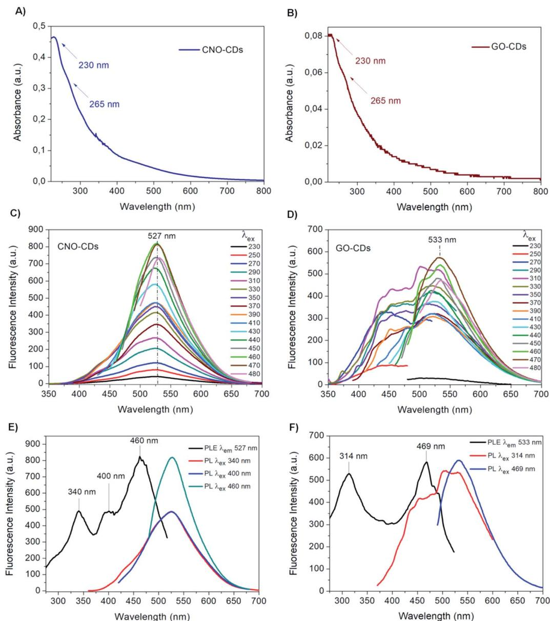
Fig. 2 UV-Vis spectra of the 1 : 10 diluted aqueous solutions of (A) CNO-CDs and (B) GO-CDs. Fluorescence emission spectra of (C) CNO-CDs and (D) GO-CDs at an increasing excitation wavelength (from 230 to 480 nm). Fluorescence excitation spectra of (E) CNO-CDs and (F) GO-CDs.
