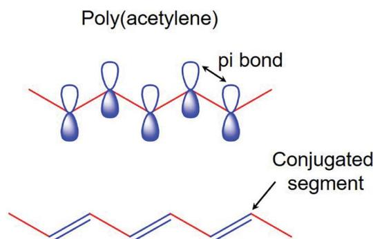
Fig. 1 The  $\pi$ -conjugated system of conducting polymers.
