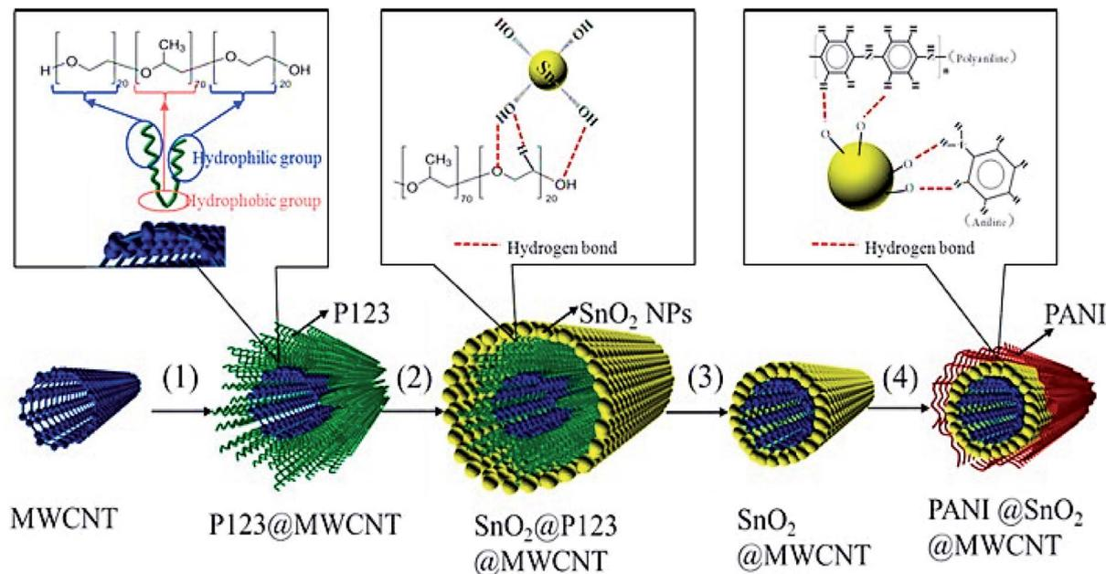
Fig. 12 The preparation of PANI@SnO<sub>2</sub>@MWCNT; steps (1)–(4) represent the dissolution, self-assembly, heating, and *in situ* polymerization. Reproduced with permission from ref. 116. Copyright 2018 Elsevier.
