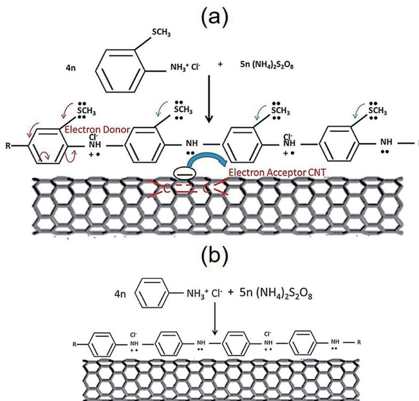
Fig. 10 The electron conjugation process of the SCH<sub>3</sub> group of (a) PMTA versus (b) PANI, accompanied by the traditional donor–acceptor state of the interaction (probable conduction mechanism). Reproduced with permission from ref. 101. Copyright 2017 Elsevier.
