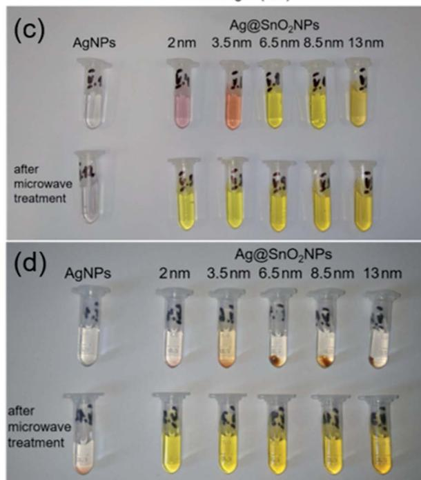
Fig. 6 Absorbance spectra of the AgNPs and AgNPs covered with SnO<sub>2</sub> in 0.1 M TBS (a) before and (b) after microwave treatment and the images of the NPs treated with 0.1 M TBS (c) for 1 h and (d) 72 h.
