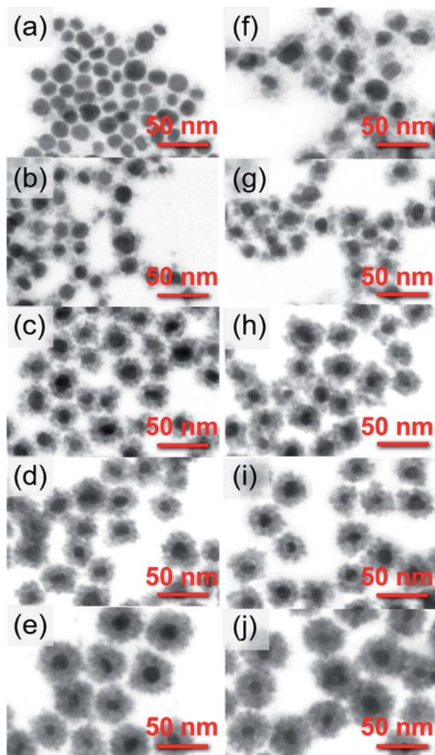
Fig. 2 STEM images of AgNPs covered with (a and f) 2, (b and g) 3.5, (c and h) 6.5, (d and i) 8.5, and (e and j) 13 nm SnO<sub>2</sub> shells (a–e) before and (f–j) after microwave treatment.
