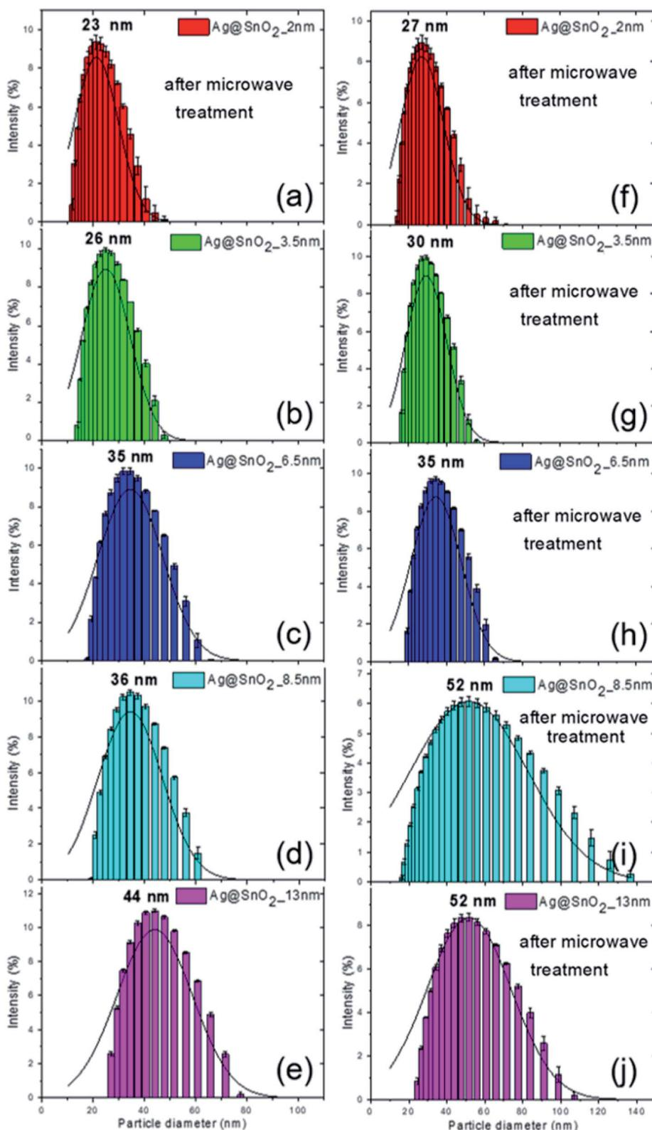
Fig. 1 The DLS size distribution by the intensity of AgNPs coverage with (a and f) 2, (b and g) 3.5, (c and h) 6.5, (d and i) 8.5, and (e and j) 13 nm SnO<sub>2</sub> shells (a–e) before and (f–j) after microwave treatment.
