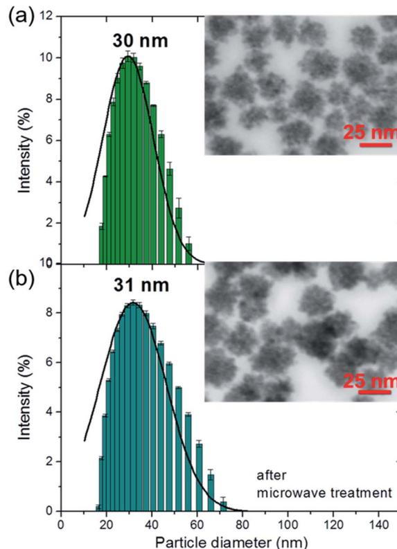
Fig. 3 DLS size distributions by the intensity and the STEM images (insets) of SnO<sub>2</sub>NPs (a) before and (b) after microwave treatment.
