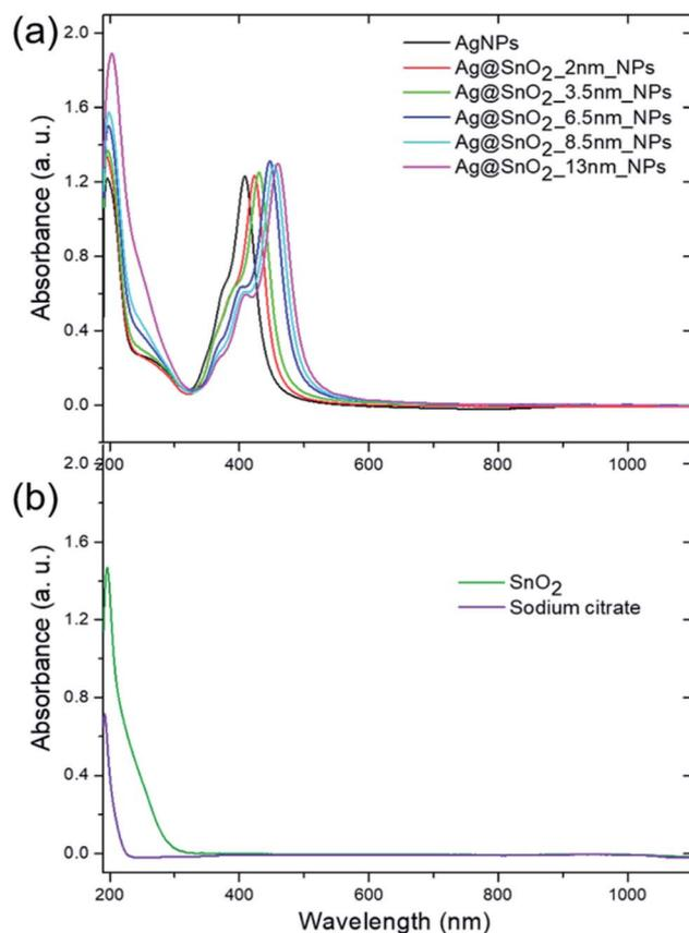
Fig. 4 Absorbance spectra of the (a) AgNPs, (a) Ag@SnO<sub>2</sub>NPs, (b) SnO<sub>2</sub>NPs and (b) sodium citrate at the same concentration as in all the optically evaluated samples of the AgNPs and Ag@SnO<sub>2</sub>NPs.
