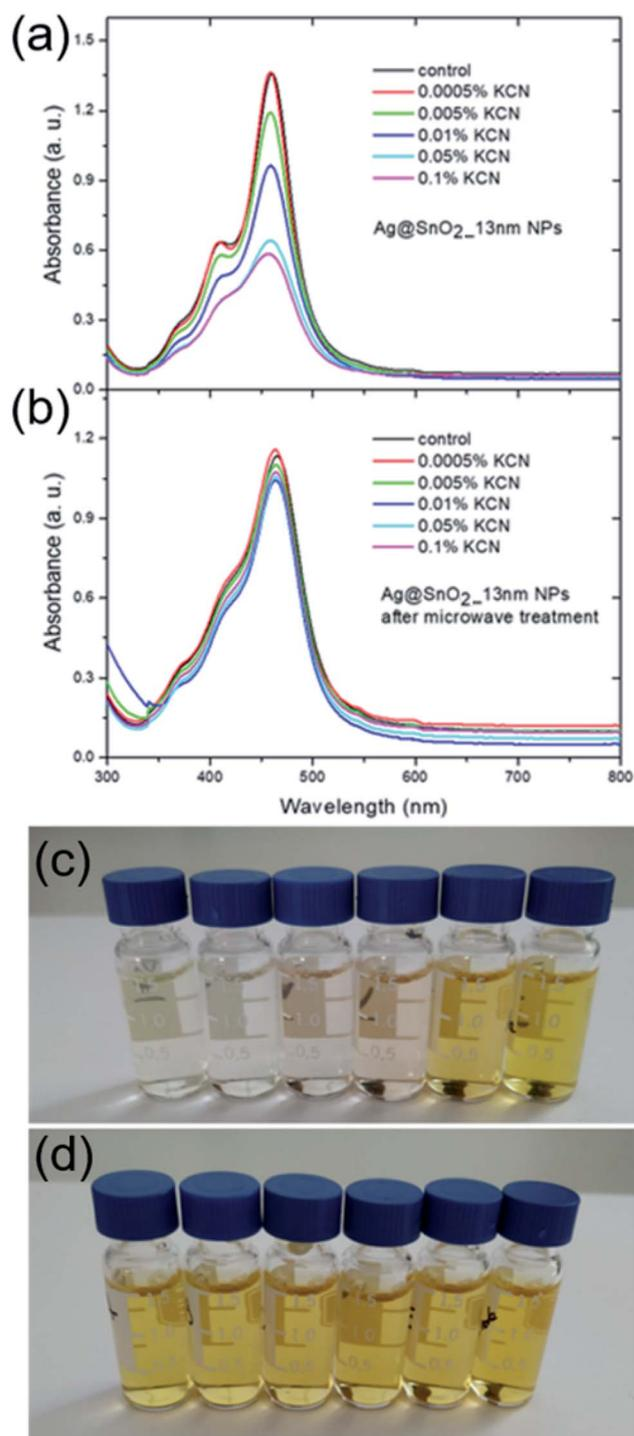
Fig. 9 (a and b) Absorbance spectra and (c and d) images of AgNPs and AgNPs covered with SnO<sub>2</sub> (13 nm) in different concentrations of KCN (a and c) before and (b and d) after microwave treatment. (c and d) Images of 13 nm Ag@SnO<sub>2</sub>NPs, from left to right, show the samples treated with 0.1, 0.05, 0.01, 0.005, and 0.0005 wt% KCN and the control sample (the as-synthesized AgNPs).
