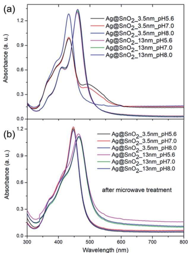
Fig. 7 The absorbance spectra of the AgNPs covered with 3.5 and 13.0 nm-thick SnO<sub>2</sub> shell (a) untreated and (b) treated with microwaves and further immersed in phosphate buffer at 0.1 M and pH of 5.6, 7.0, and 8.0.
