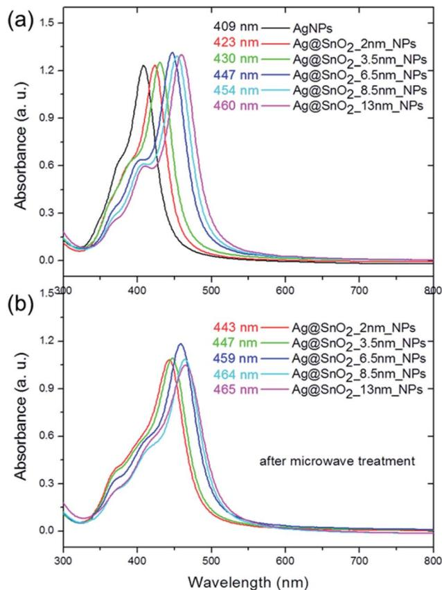
Fig. 5 The absorbance spectra of Ag@SnO<sub>2</sub>NPs (a) before and (b) after microwave treatment.
