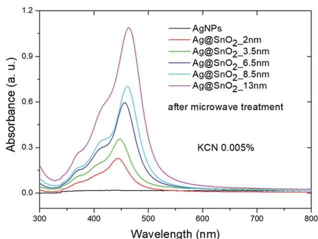
Fig. 8 Absorbance spectra of AgNPs and Ag@SnO<sub>2</sub>NPs after microwave treatment in 0.005 wt% KCN.
