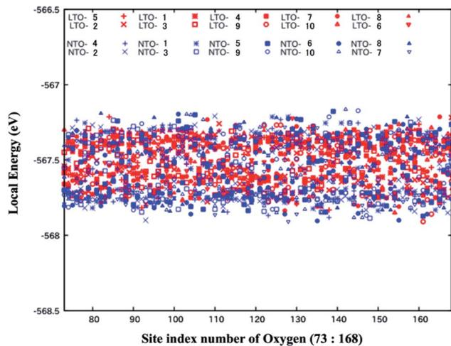
Fig. 7 Local energy of oxygen atoms for the optimized top ten stable structures of  $\text{Li}_4\text{Ti}_5\text{O}_{12}$  and  $\text{Na}_3\text{LiTi}_5\text{O}_{12}$ . LTO-1 and NTO-1 (LTO-10 and NTO-10) indicate the most stable (the 10-th stable) models. The abscissa is the site index of oxygen (73 to 168) of the total 168 sites in the superlattice of  $\text{Li}_4\text{Ti}_5\text{O}_{12}$  and  $\text{Na}_3\text{LiTi}_5\text{O}_{12}$  used in the present study.
