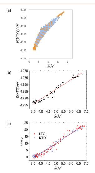
Fig. 3 Total energy E(NTO) of  $Na_3LiTi_5O_{12}$  as a function of S for (a) 8444 non-optimized structures and (b) 58 optimized structures whose initial positions are indicated with orange squares in (a). (c) Energy difference from the most stable structure ( $\Delta E$ ) as a function of S for the optimized structures of  $Li_4Ti_5O_{12}$  and  $Na_3LiTi_5O_{12}$ .
