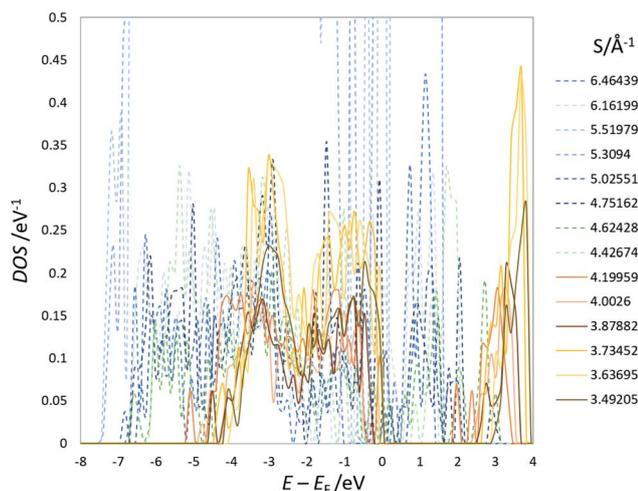
Fig. 4 An example of the DOS of optimized structures of Na<sub>3</sub>LiTi<sub>5</sub>O<sub>12</sub> (others are shown in the ESI†).  $E_f$  represents the Fermi energy.
