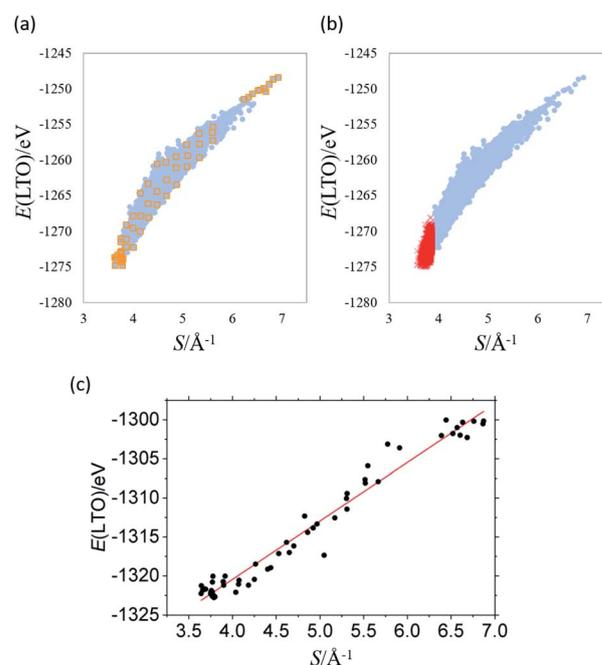
Fig. 1 Total energy  $E(\text{LTO})$  of  $\text{Li}_4\text{Ti}_5\text{O}_{12}$  as a function of the sum of the inverse distance between Li in the 16d sites  $S$  for (a) 8444 non-optimized structures, (b) additional 5000 structures (red cross) overlaid on (a), and (c) 58 optimized structures whose initial positions are indicated with orange squares in (a).
