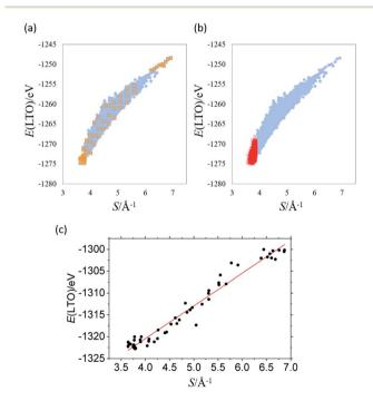
Fig. 1 Total energy E(LTO) of  $Li_4Ti_5O_{12}$  as a function of the sum of the inverse distance between Li in the 16d sites S for (a) 8444 non-optimized structures, (b) additional 5000 structures (red cross) overlaid on (a), and (c) 58 optimized structures whose initial positions are indicated with orange squares in (a).
