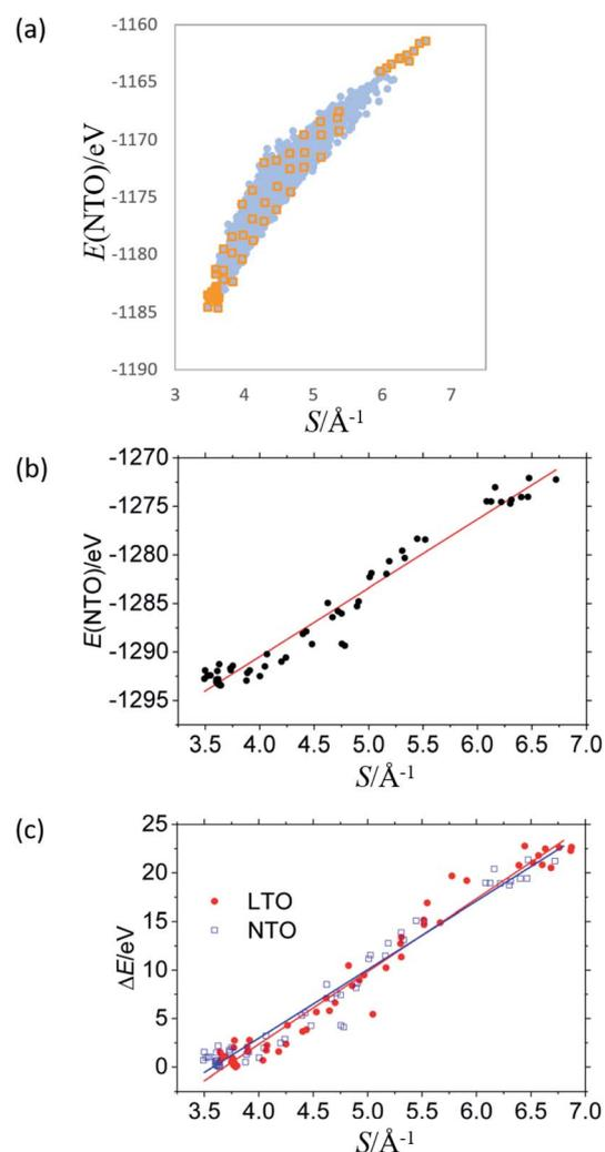
Fig. 3 Total energy  $E(\text{NTO})$  of  $\text{Na}_3\text{LiTi}_5\text{O}_{12}$  as a function of  $S$  for (a) 8444 non-optimized structures and (b) 58 optimized structures whose initial positions are indicated with orange squares in (a). (c) Energy difference from the most stable structure ( $\Delta E$ ) as a function of  $S$  for the optimized structures of  $\text{Li}_4\text{Ti}_5\text{O}_{12}$  and  $\text{Na}_3\text{LiTi}_5\text{O}_{12}$ .
