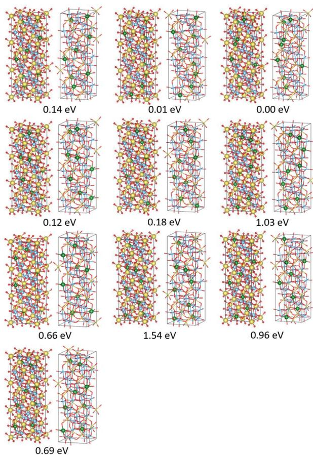
Fig. 6 Perspective views of the optimized top ten stable structures and their  $\Delta E$  values (the energy difference in the total energy from the most stable structure) for  $\text{Na}_3\text{LiTi}_5\text{O}_{12}$ . In the left panels, spheres in yellow, green, blue, and red represent Na, Li, Ti, and O atoms, respectively. In right panels, the Li atoms in the 16d sites are shown as the green spheres, and the other atoms are shown as the sticks.
