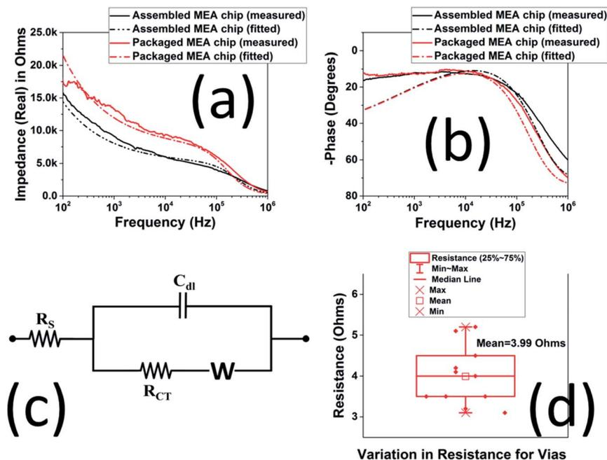
Fig. 6 (a) Impedance (real) spectra of the assembled device, packaged device with 3D printed frame and fitted plot as per Randles equivalent circuit; (b) phase spectra of the assembled device, packaged device with 3D printed frame and fitted plot as per (c) Randles' equivalent circuit used for circuit fitting and extraction; (d) box plot of the DC resistance of the vias after silver ink casting process.
