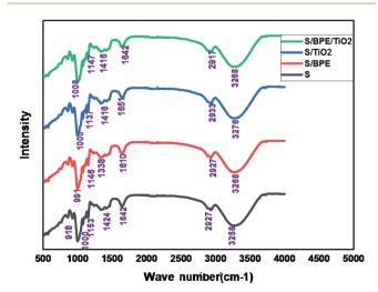
Fig. 3 FTIR spectra of S, S/BPE, S/TiO<sub>2</sub> and S/BPE/TiO<sub>2</sub> films.
