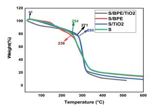
Fig. 5 TG curves of S, S/BPE, S/TiO<sub>2</sub> and S/BPE/TiO<sub>2</sub> films.
