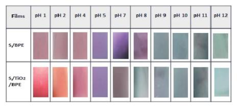
Fig. 6 Visual aspect colour of the S/BPE and S/BPE/ $TiO_2$  starch pH indicator films with butterfly pea extract after immersion in buffer solutions having different pH values (1–12).
