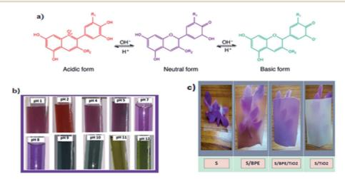
Fig. 1 (a) Chemical diagram of colour-changing anthocyanin pH reaction<sup>37</sup> (b) colour variations of BPE in different buffer solutions (c) photographs of starch films showing the transparency.
