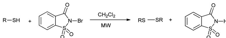
Scheme 36 Oxidation of thiols to the disulfides.
