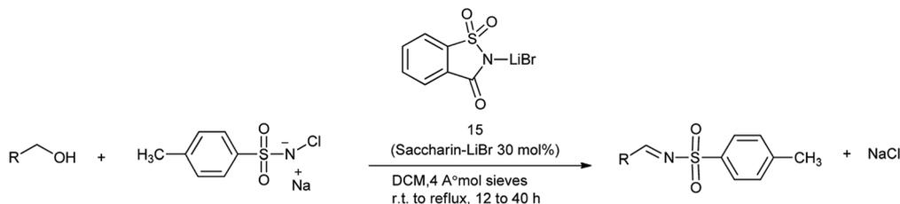
Scheme 90 Synthesis of *N*-tosylimines directly from alcohols.
