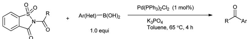
Scheme 75 Pd-catalyzed acylative Suzuki coupling of amides.
