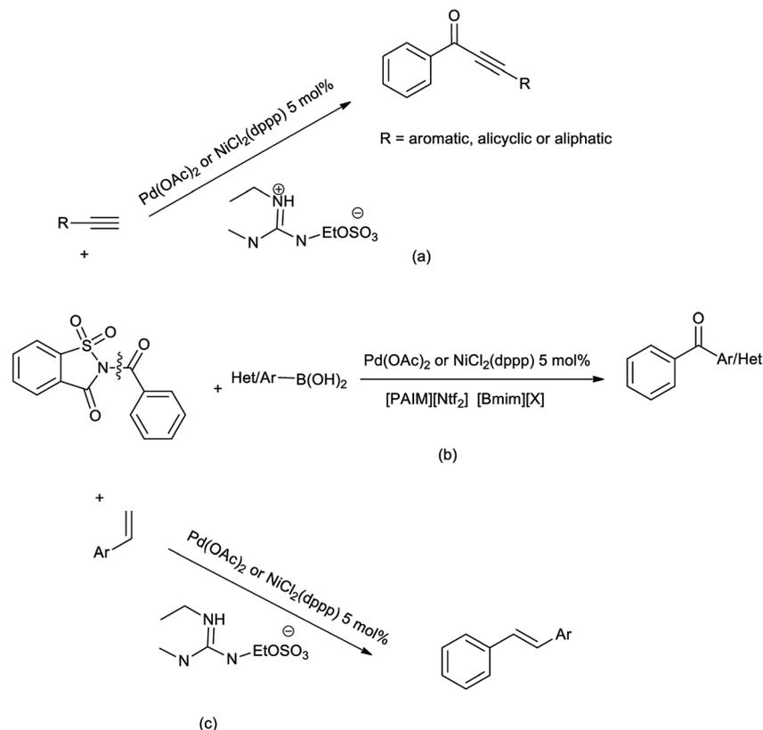
Scheme 79 (a) *trans*-Benzoylation Sonogashira cross-coupling in GIL using *N*-benzoylsaccharin, (b) *trans*-benzoylation Suzuki cross-coupling using *N*-benzoylsaccharin, and (c) decarbonylative Heck coupling in GIL using *N*-benzoylsaccharin.
