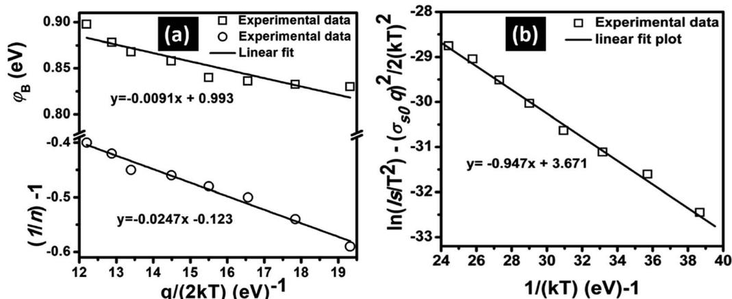
Fig. 4 (a) The zero-bias apparent barrier heights extracted from  $I$ - $V$  analysis plotted against the  $q/2kT$  and ideality factor versus  $q/2kT$  according to the GD of the BHs and (b) the modified Richardson plots  $\ln(I_s/T^2) - 0.5\sigma_s^2 q^2/(kT)^2$  vs.  $1/kT$  according to the GD of the BHs.
