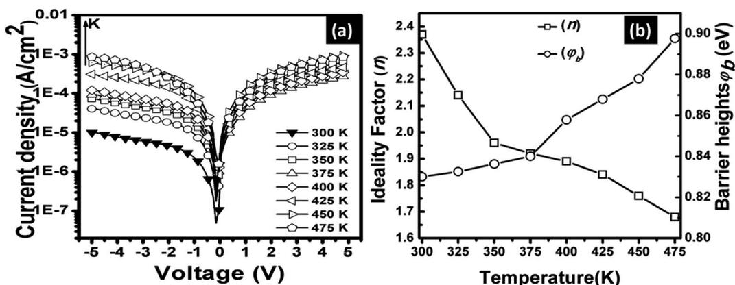
Fig. 2 (a) Temperature-dependent  $J$ - $V$  semi log plot for n-GaN/p-Si heterojunction and (b) the variations of ideality factor and barrier height as a function of temperature obtained from TE for GaN/Si heterojunction.
