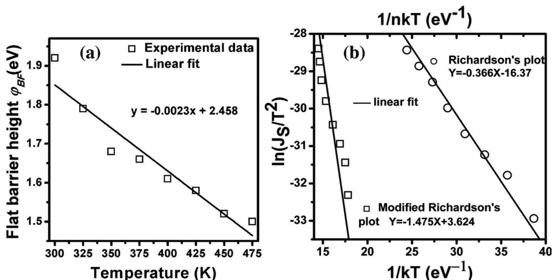
Fig. 3 (a) Variation of flat band barrier heights as a function of temperature for n-GaN/p-Si heterojunction and (b) conventional Richardson plot,  $\ln I_s/T^2$  vs.  $1/kT$  and "modified" Richardson's plot  $\ln I_s/T^2$  vs.  $1/nkT$  for the fabricated heterojunction.
