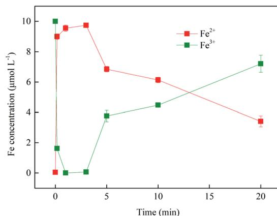
Fig. 2 Variation in concentrations of Fe<sup>2+</sup> and Fe<sup>3+</sup> during SMX removal. Experimental conditions: [BS]<sub>0</sub> = 100 μmol L<sup>-1</sup>, [Fe<sup>3+</sup>]<sub>0</sub> = 10 μmol L<sup>-1</sup>, [SMX]<sub>0</sub> = 1 μmol L<sup>-1</sup>, pH<sub>0</sub> = 4.0, T = 25 °C.
