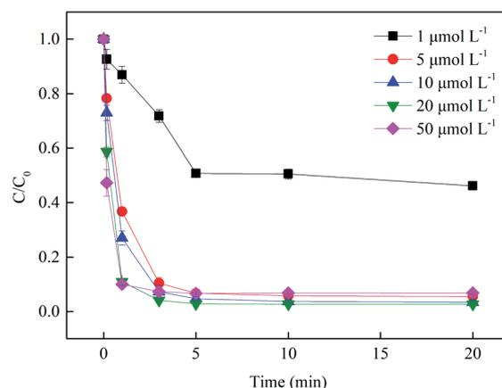
Fig. 6 Effect of  $\text{Fe}^{3+}$  dosage on SMX removal. Experimental conditions:  $[\text{BS}]_0 = 100 \mu\text{mol L}^{-1}$ ,  $[\text{SMX}]_0 = 1 \mu\text{mol L}^{-1}$ ,  $\text{pH}_0 = 4.0$ ,  $T = 25 \text{ }^\circ\text{C}$ .
