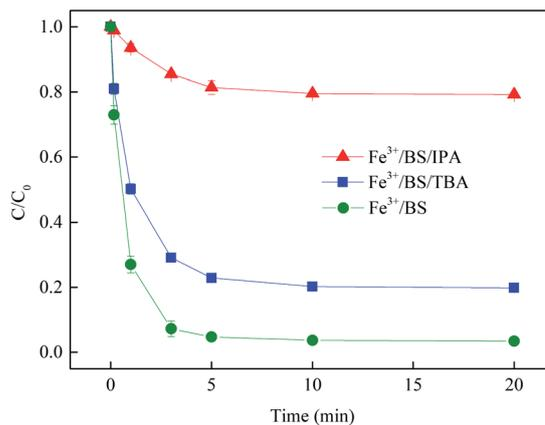
Fig. 1 Effect of radical scavenger on SMX removal. Experimental conditions: [BS]<sub>0</sub> = 100 μmol L<sup>-1</sup>, [Fe<sup>3+</sup>]<sub>0</sub> = 10 μmol L<sup>-1</sup>, [SMX]<sub>0</sub> = 1 μmol L<sup>-1</sup>, [IPA]<sub>0</sub> = [TBA]<sub>0</sub> = 1000 μmol L<sup>-1</sup>, pH<sub>0</sub> = 4.0, T = 25 °C.
