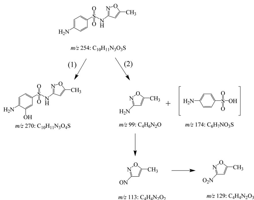
Fig. 3 Possible removal pathways of SMX by Fe<sup>3+</sup>/BS: (1) hydroxylation and (2) bond cleavage.
