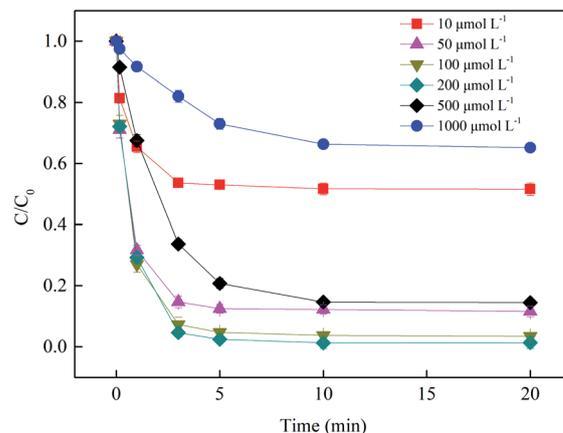
Fig. 5 Effect of BS dosage on SMX removal. Experimental conditions:  $[\text{SMX}]_0 = 1 \mu\text{mol L}^{-1}$ ,  $[\text{Fe}^{3+}]_0 = 10 \mu\text{mol L}^{-1}$ ,  $\text{pH}_0 = 4.0$ ,  $T = 25 \text{ }^\circ\text{C}$ .
