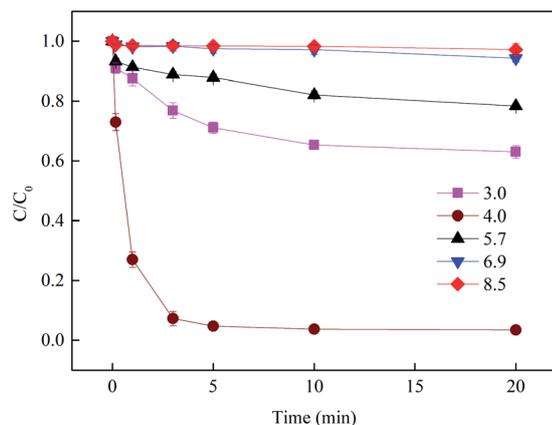
Fig. 4 Effect of initial pH on SMX removal. Experimental conditions:  $[\text{Fe}^{3+}]_0 = 10 \mu\text{mol L}^{-1}$ ,  $[\text{BS}]_0 = 100 \mu\text{mol L}^{-1}$ ,  $[\text{SMX}]_0 = 1 \mu\text{mol L}^{-1}$ ,  $T = 25 \text{ }^\circ\text{C}$ .
