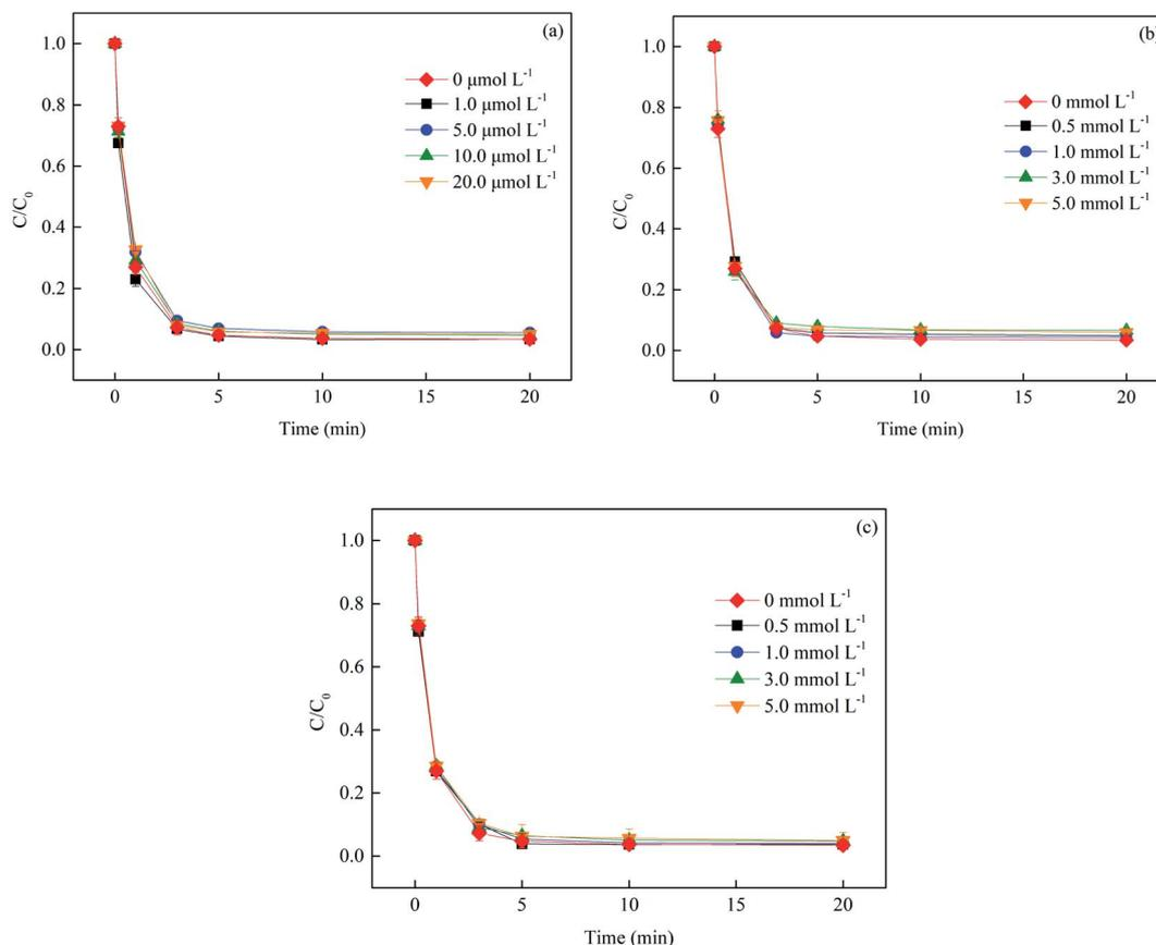
Fig. 9 Effect of Cu<sup>2+</sup> (a), Ca<sup>2+</sup> (b), and Mg<sup>2+</sup> (c) on SMX removal. Experimental conditions: [BS]<sub>0</sub> = 100 μmol L<sup>-1</sup>, [Fe<sup>3+</sup>]<sub>0</sub> = 10 μmol L<sup>-1</sup>, [SMX]<sub>0</sub> = 1 μmol L<sup>-1</sup>, pH<sub>0</sub> = 4.0, T = 25 °C.
