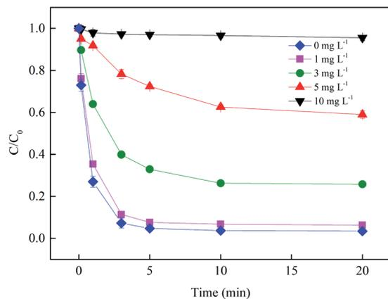
Fig. 7 Effect of NOM on SMX removal. Experimental conditions:  $[BS]_0 = 100 \mu\text{mol L}^{-1}$ ,  $[\text{Fe}^{3+}]_0 = 10 \mu\text{mol L}^{-1}$ ,  $[\text{SMX}]_0 = 1 \mu\text{mol L}^{-1}$ ,  $\text{pH}_0 = 4.0$ ,  $T = 25^\circ\text{C}$ .
