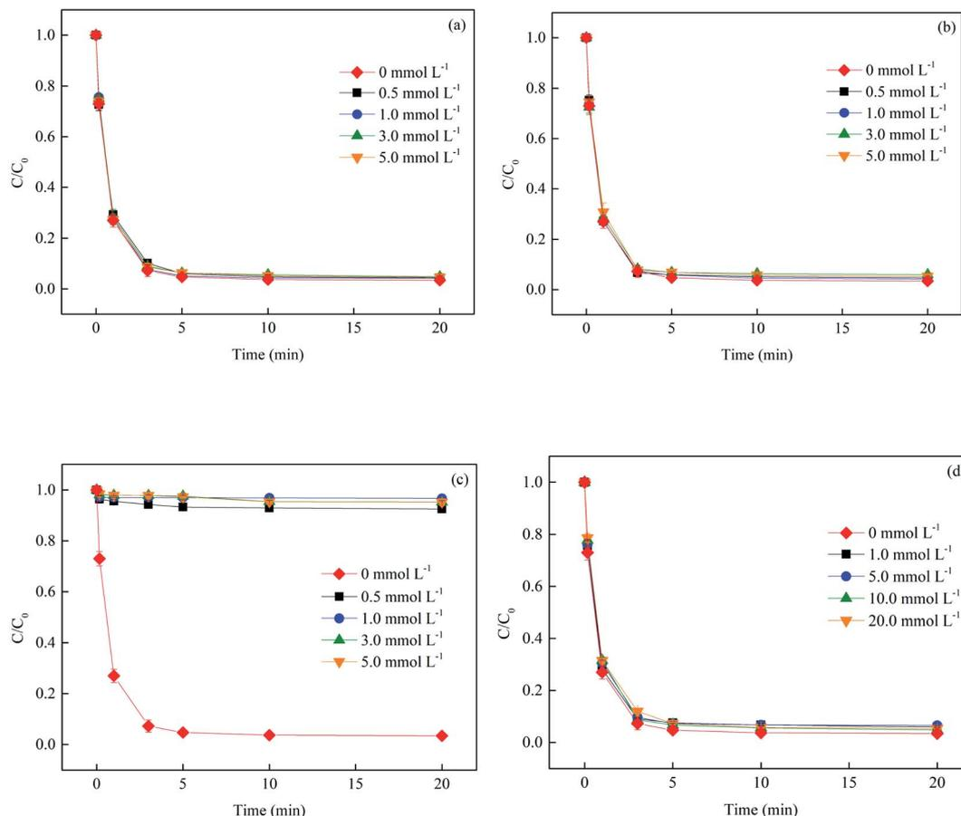
Fig. 8 Effect of  $\text{SO}_4^{2-}$  (a),  $\text{NO}_3^-$  (b),  $\text{HCO}_3^-$  (c) and  $\text{Cl}^-$  (d) on SMX removal. Experimental conditions:  $[BS]_0 = 100 \mu\text{mol L}^{-1}$ ,  $[\text{Fe}^{3+}]_0 = 10 \mu\text{mol L}^{-1}$ ,  $[\text{SMX}]_0 = 1 \mu\text{mol L}^{-1}$ ,  $\text{pH}_0 = 4.0$ ,  $T = 25^\circ\text{C}$ .
