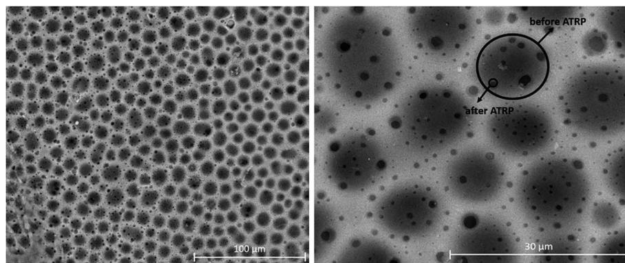
Fig. 6 SEM images of PVC-I-g-PAA (B) membrane.
