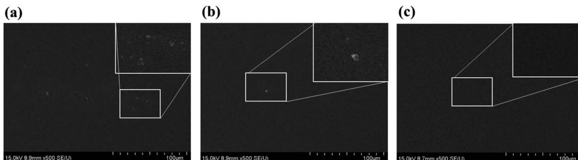
Fig. 2 SEM images show states of the PDLC mixtures: (a) after stirring at room temperature, (b) after stirring at the hot plate, and (c) after stirring at the hot plate and under vacuum. The insets are the magnified images showing any undissolved clusters of nanoparticles.
