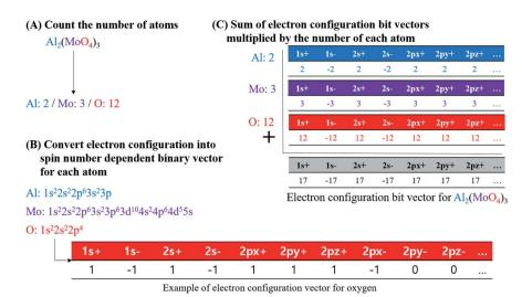
Fig. 4 Procedure of calculating the electronic configuration bit vectors for inorganic compounds, taking  $Al_2(MoO_4)_3$  as an example molecule.
