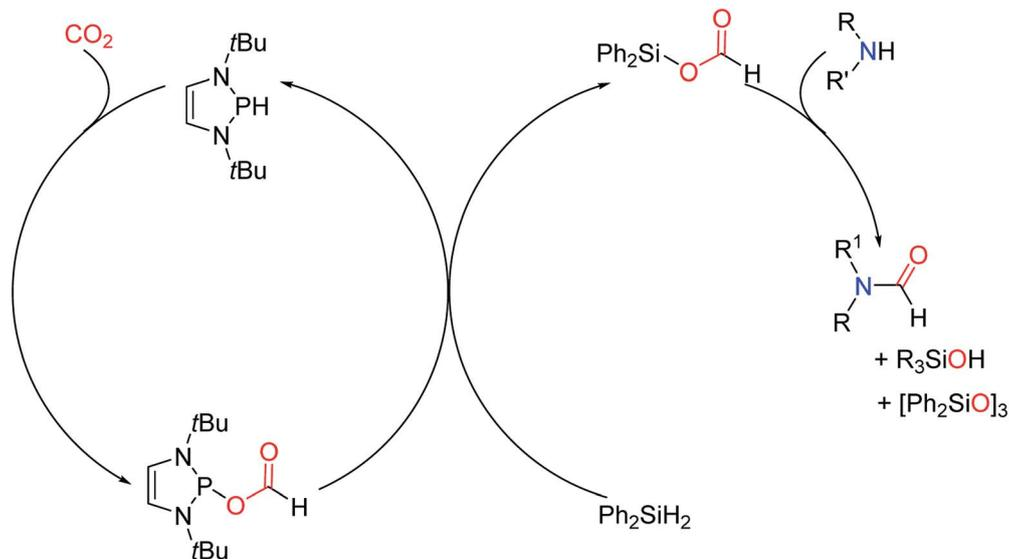
Scheme 29 The mechanism of the 1,3,2-diazaphospholene catalytic *N*-formylation of amines with CO<sub>2</sub> and Ph<sub>2</sub>SiH<sub>2</sub>.<sup>37</sup>
