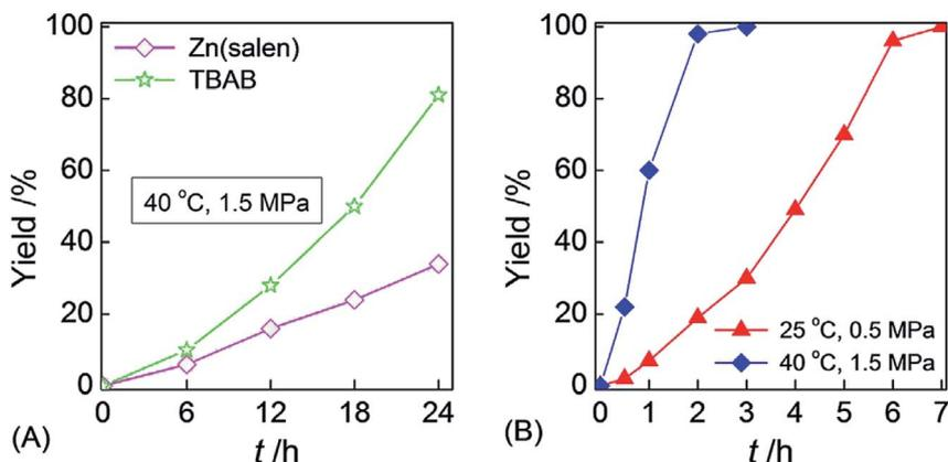
Fig. 4 Kinetic curves from the *N*-formylation reaction of *N*-methylaniline, CO<sub>2</sub>, and PhSiH<sub>3</sub> catalyzed by the (A) one-component Zn(salen) or (B) Zn(salen)/TBAB bicomponent catalyst. Reaction conditions: 10 mL stainlesssteel autoclave, *N*-methylaniline (1.0 mmol), PhSiH<sub>3</sub> (1.0 mmol), Zn(salen) (0.5 mol%), TBAB (1.0 mol%), CO<sub>2</sub> pressure (0.5 MPa or 1.5 MPa), reaction temperature (25 °C or 40 °C).<sup>96</sup>
