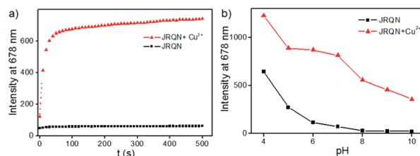
Fig. 4 (a) Time-dependence fluorescence intensity of **JRQN** (10  $\mu\text{M}$ ) upon addition of 100  $\mu\text{M}$   $\text{Cu}^{2+}$ ; (b) fluorescence intensity of **JRQN** (10  $\mu\text{M}$ ) as a function of pH value in the absence/presence of  $\text{Cu}^{2+}$  (100  $\mu\text{M}$ ); the conditions: HEPES buffer (10 mM, pH = 7.4, containing 20%  $\text{CH}_3\text{CN}$ ),  $\lambda_{\text{ex}}$  = 580 nm, slit = 5/5 nm.
