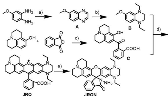
Scheme 1 Synthesis of dye **JRQ** and probe **JRQN**. Reagents and conditions: (a) succinaldehyde, CH<sub>3</sub>CN, 60 °C, overnight; (b) NaBH<sub>4</sub>, toluene, AcOH, 5 °C to reflux, 5 h; (c) toluene, reflux, overnight; (d) CH<sub>3</sub>SO<sub>3</sub>H, 80 °C, 8 h; (e) NH<sub>2</sub>NH<sub>2</sub>, MeOH, 50 °C, 6 h.
