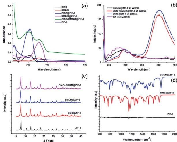
Fig. 2 (a) UV-vis spectra of ethanolic solutions of void ZIF-8, OMC@ZIF-8, BMDM@ZIF-8 and OMC + BMDM@ZIF-8. For each OMC-containing sample the OMC concentration was  $5 \mu\text{g mL}^{-1}$ , and for each BMDM-containing sample, the BMDM concentration was  $5 \mu\text{g mL}^{-1}$ . (b) Fluorescence spectra under 228 nm excitation (c) powder XRD patterns and (d) FTIR spectra of ZIF-8, OMC@ZIF-8, and BMDM@ZIF-8 nanocapsules.
