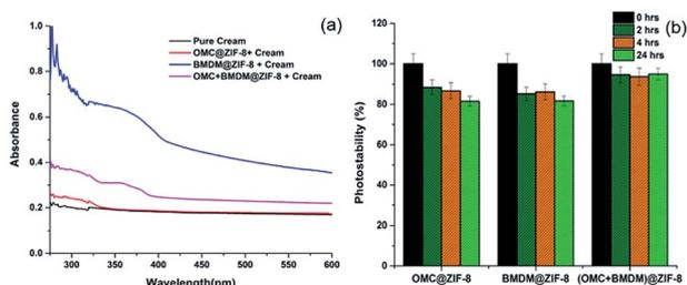
Fig. 4 (a) UV-vis spectra of pure cream (Aveeno body lotion) and OMC@ZIF-8, BMDM@ZIF-8, and OMC + BMDM@ZIF-8 nanocapsules after mixing with cream (b) photostability of void ZIF-8 and OMC@ZIF-8, BMDM@ZIF-8, and OMC + BMDM@ZIF-8 after 0, 2, 4 and 24 hours.
