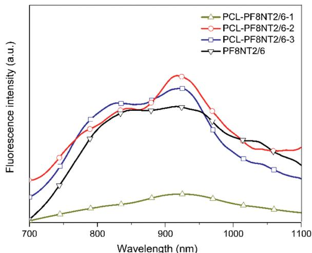
Fig. 1 Fluorescence spectra of free PF8NT2/6 NIR dye ( $0.05 \text{ mg mL}^{-1}$  in chloroform) and PCL-PF8NT2/6 nanoparticles ( $0.05 \text{ mg mL}^{-1}$  in DI water) prepared using different surfactants ( $\lambda_{\text{ex}} = 610 \text{ nm}$ ).
