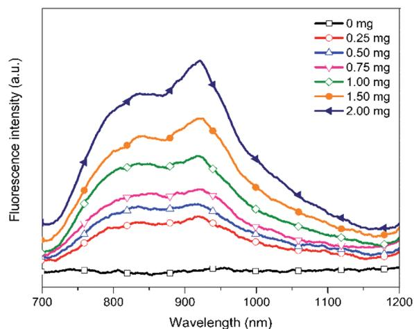
Fig. 3 Fluorescence intensity of the PCL-PF8NT2/6-3 nanoparticles in aqueous media at different dye concentrations.
