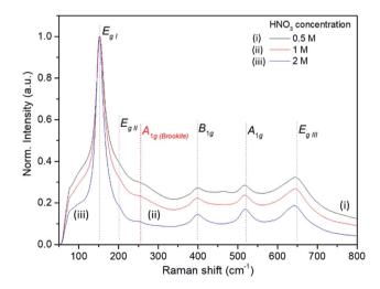
Fig. 5 Raman spectra of selected as-made FMS  $TiO_2$  sub-microspheres (80 mM TTIP) as a function of acid concentration, using: (i) 0.5 M, (ii) 1 M and (iii) 2 M  $HNO_3$  respectively. The spectra are normalised against the  $E_{\alpha,l}$  mode peak intensity.
