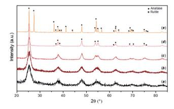
Fig. 1 PXD patterns for as-made FMS samples (2 M HNO $_3$ /160 mM TTIP; 1 min MW treatment) calcined for 3 h in air at different temperatures showing: (a) as-prepared sample; samples after heating to: (b) 300 °C, (c) 400 °C, (d) 500 °C and (e) 600 °C respectively. Anatase (squares) and rutile (asterisks) reflections are indicated on the patterns for samples heated at 500 °C and 600 °C respectively.
