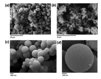
Fig. 2 SEM images showing examples of as-made FMS  $TiO_2$  sub-microspheres using ethanol as a solvent with: (a) 0.5 M  $HNO_3/320$  mM TTIP; (b) 1 M  $HNO_3/80$  mM TTIP. (c and d) HR-SEM images of FMS- $TiO_2$  sub-microspheres produced using 1 M  $HNO_3/160$  mM TTIP.
