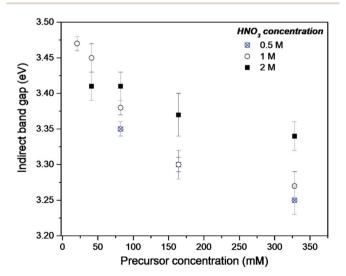
Fig. 9 Indirect band gap values for as-made FMS-TIO<sub>2</sub> sub-microspheres as a function of TTIP concentration using 0.5 M (crosses/circles), 1 M (open circles) or 2 M (filled squares) HNO<sub> $\frac{\pi}{2}$ </sub> respectively.
