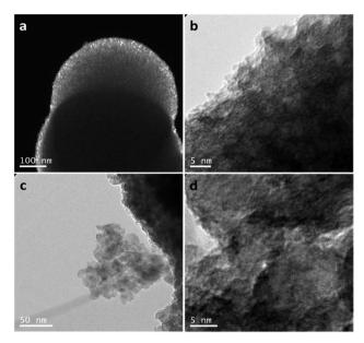
Fig. 3 TEM images of as-made FMS-TiO $_2$  sub-microspheres synthesised in absolute ethanol with 2 M HNO $_3$ ,/160 mM TTIP: (a) dark field image of the spheres; (b) bright field image showing the detail of the sphere surface at high magnification; (c) cluster of primary NPs dissociated from a sub-microsphere after calcination at 500 °C for 3 h (10 °C min $^{-1}$ ) and (d) detail of the lattice fringes observable at high magnification after calcination at 500 °C for 3 h (10 °C min $^{-1}$ ).
