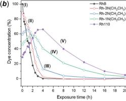
Fig. 11 (a) Degradation curves for the 5 degrees of N-ethylation of the Rhodamine molecule (where (I) RhB contains 4 N-ethyl groups and (V) Rh110 contains none) for: (a) P25 and (b) as-made FMS TiO<sub>2</sub> sub-microspheres under visible light irradiation; (I) RhB, (II) Rh-3N-Et, (III) Rh-2N-Et, (IV) Rh-1N-Et, (V) Rh110.
