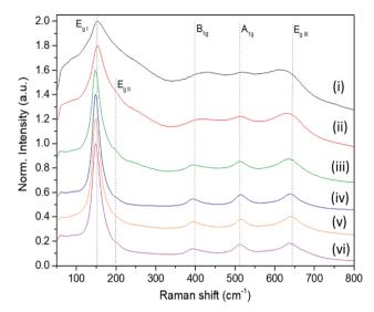
Fig. 4 Raman spectra of as-made FMS  $TiO_2$  sub-microspheres (1 M HNO<sub>3</sub>) as a function of the TTIP concentration, using: (i) 20 mM, (ii) 40 mM, (iii) 80 mM, (vi) 160 mM, (v) 320 mM and (vi) 650 mM TTIP, respectively. The spectra are normalised against the  $E_{g,I}$  mode peak intensity.
