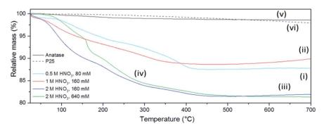
Fig. 7 Thermogravimetric (TG) profiles of selected as-prepared FMS-TiO<sub>2</sub> samples (1 min MW irradiation) synthesised with (i) 0.5 M HNO<sub>3</sub>/80 mM TTIP, (ii) 1 M HNO<sub>3</sub>/160 mM TTIP, (iii) 2 M HNO<sub>3</sub>/160 mM TTIP, (iv) 2 M HNO<sub>3</sub>/640 mM TTIP in comparison to (v) commercial anatase and (vi) Aeroxide® P25 respectively.
