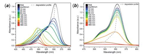
Fig. 10 Rhodamine UV-Vis absorbance spectra using: (a) as-made FMS  $TiO_2$  sub-microspheres (2 M HNO<sub>3</sub> conc. and 320 mM precursor conc.) and (b) P25 as a catalyst for its degradation under visible light. The dashed trend line indicates the shift in the maximum of the principal peak in each spectrum.
