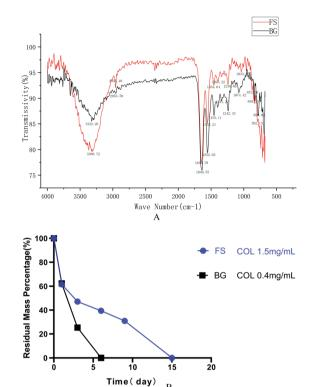
(A) FTIR; (B) degradation rate in vitro
