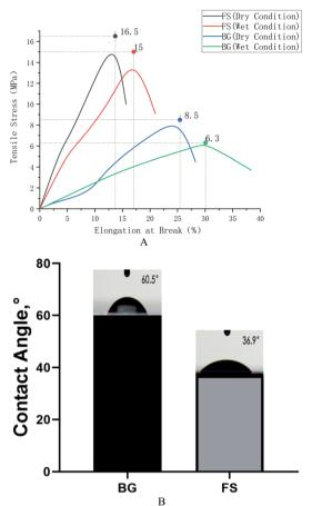
Fig. 3 (A) Tensile strength testing; (B) water contents
