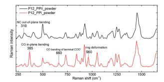
Fig. 4 Raman spectra of P12 PPI (lower) and PPII (top) powders.
