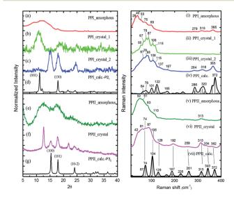
Fig. 1 ((a)–(g)) powder X-ray curves and calculated (black, (d), (g)) using PPI  $P2_1$  and PPII  $P3_2$  crystal data, and ((i)–(vii)) low-wavenumber Raman spectra of poly-L-proline I and II with simulated Raman spectra (black, (iv), (vii)) using CRYSTAL 17 at the B3LYP/6-31G(d,p) level with the coupled-perturbed Kohn–Sham scheme.
