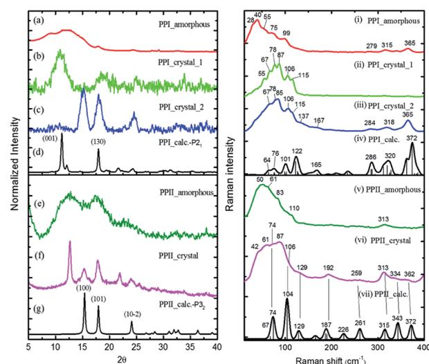
Fig. 1 ((a)–(g)) powder X-ray curves and Raman spectra (black, (d), (g)) using PPI  $P2_1$  and PPII  $P3_2$  crystal data, and ((i)–(vii)) low-wavenumber Raman spectra of poly-L-proline I and II with simulated Raman spectra (black, (iv), (vii)) using CRYSTAL 17 at the B3LYP/6-31G(d,p) level with the coupled-perturbed Kohn–Sham scheme.
