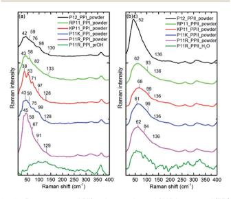
Fig. 3 Raman curves of P12 series powder and P11R in propanol (PPI) and in aqueous solution (PPII), respectively for (a) PPI and (b) PPII. The intensity is normalized to the 365 and 310 cm $^{-1}$  bands for PPI and PPII, respectively for the powder samples.
