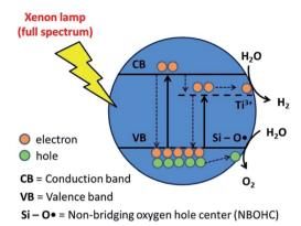
Fig. 8 Schematic mechanism of photocatalytic water splitting on 9Ti-1Si-H-UV in the presence of Ti<sup>3+</sup> and NBOHC defects.
