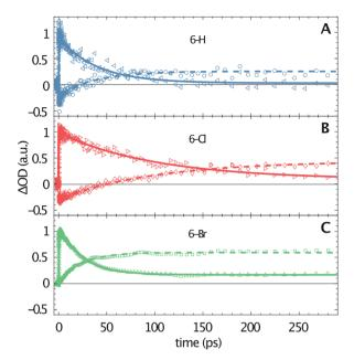
Fig. 3 Temporal evolution of 6-H (A), 6-Cl (B) and 6-Br (C) in acetonitrile after excitation at 330 nm (data points, calculated lines). Time-scans measured close to the  $\rm S_1$  absorption maximum at 640 nm (triangles, solid lines) and at 465 nm (close to the maximum of TTA, circles, dashed lines). The signal amplitudes are normalized to the respective maximum at 640 nm.
