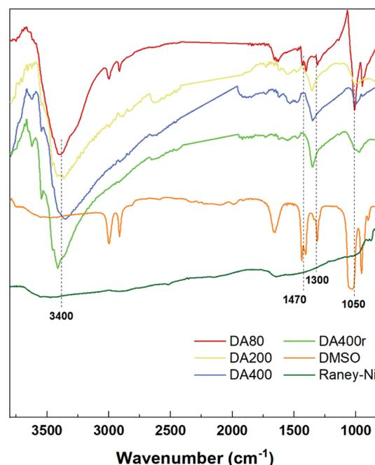
Fig. 1 FT-IR spectra for different catalysts.
