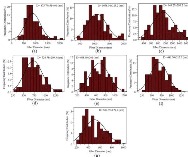
Fig. 6 (a–g) Fiber diameter distributions of electrospun nanofibers of PVDF/BaTiO<sub>3</sub> solution with PVDF concentration of 25 wt% and various BaTiO<sub>3</sub> concentrations of 6 wt%, 12 wt%, 18 wt%, 20 wt%, 22 wt%, 24 wt% and 26 wt%, respectively.
