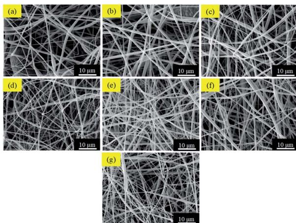
Fig. 5 (a–g) SEM images of produced electrospun nanofiber from PVDF/BaTiO<sub>3</sub> solution with PVDF concentration of 25 wt% and various BaTiO<sub>3</sub> concentrations of 6 wt%, 12 wt%, 18 wt%, 20 wt%, 22 wt%, 24 wt% and 26 wt%, respectively.
