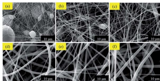
Fig. 1 (a–f) SEM images of electrospun nanofibers with different PVDF concentration of 19, 21, 23, 25, 27, 29 wt%, respectively.
