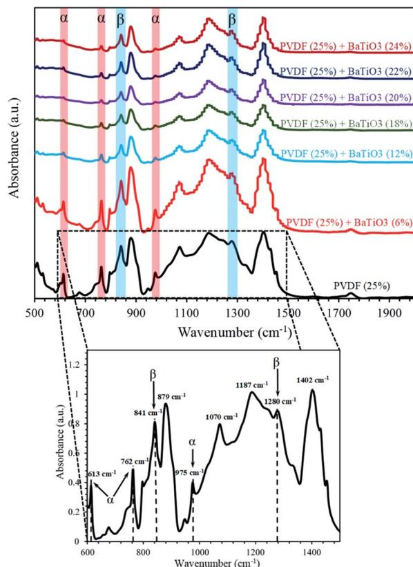
Fig. 7 FTIR results of electrospun nanofiber mats made of PVDF and PVDF/BaTiO<sub>3</sub> with various concentrations of BaTiO<sub>3</sub>. A magnified spectra for pure PVDF is shown with more details.
