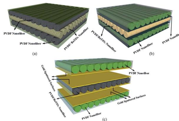
Fig. 10 (PVDF)–(PVDF/BaTiO<sub>3</sub>)–(PVDF) three layer electrospun nanocomposite, (a) continuously sprayed, (b) separately sprayed and (c) separately sprayed with gold sputtered surfaces.
