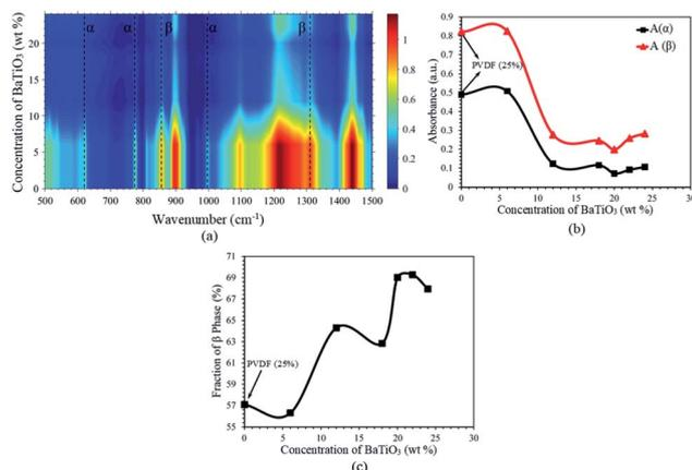
Fig. 8 (a) FTIR spectra of the PVDF/BaTiO<sub>3</sub> electrospun nanofiber as functions of wavenumber and concentration of BaTiO<sub>3</sub> nanoparticles, (b) variations of absorbance peaks of  $\alpha$  and  $\beta$  phases as a function of BaTiO<sub>3</sub> concentrations, and (c) variations of fraction of  $\beta$  as a function of BaTiO<sub>3</sub> concentrations. Zero concentration stands for PVDF 25 wt% in all plots.
