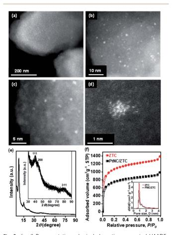
Fig. 2 (a-d) Representative spherical aberration-corrected HAADF-STEM images of PtNC/ZTC at various magnifications. (e) XRD pattern of PtNC/ZTC and (f) Ar adsorption-desorption isotherms of ZTC and PtNC/ZTC. Inset in (e) shows a 30 times magnified high-angle region of XRD of PtNC/ZTC. Inset in (f) shows the pore size distributions of the ZTC and PtNC/ZTC.
