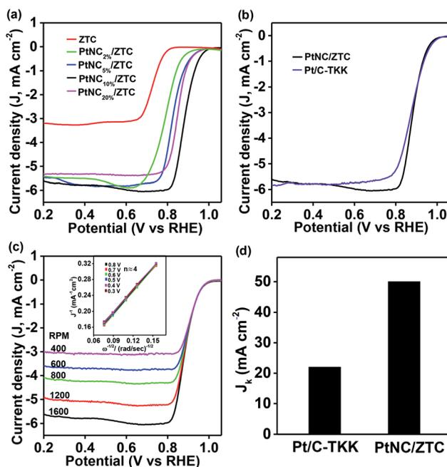
Fig. 3 (a) RDE ORR polarization curves of PtNC/ZTC with different mass loading of Pt. (b) Comparison of PtNC/ZTC (PtNC<sub>10%</sub>/ZTC) with commercial Pt/C-TKK at the same loading of  $40 \mu\text{g}_{\text{Pt}} \text{ cm}^{-2}$ . (c) RDE ORR polarization curves of PtNC/ZTC at different rotation speeds. Inset in (c) shows the corresponding K–L plots at different rotation potentials. (d) Represents the kinetic current density values of Pt/C-TKK and PtNC/ZTC at the potential of 0.8 V vs. RHE.
