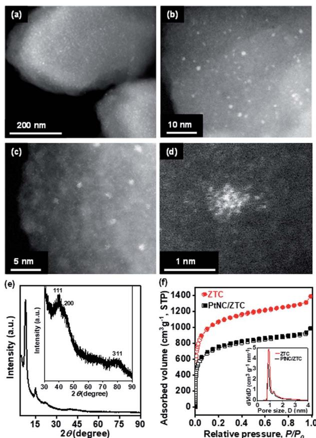
**Fig. 2** (a–d) Representative spherical aberration-corrected HAADF-STEM images of PtNC/ZTC at various magnifications. (e) XRD pattern of PtNC/ZTC and (f) Ar adsorption–desorption isotherms of ZTC and PtNC/ZTC. Inset in (e) shows a 30 times magnified high-angle region of XRD of PtNC/ZTC. Inset in (f) shows the pore size distributions of the ZTC and PtNC/ZTC.
