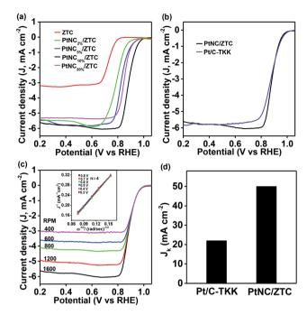
Fig. 3 (a) RDE ORR polarization curves of PtNC/ZTC with different mass loading of Pt. (b) Comparison of PtNC/ZTC (PtNC $_{10\%}$ /ZTC) with commercial Pt/C-TKK at the same loading of 40  $\mu g_{Pt}$  cm $^{-2}$ . (c) RDE ORR polarization curves of PtNC/ZTC at different rotation speeds. Inset in (c) shows the corresponding K–L plots at different potentials. (d) Represents the kinetic current density values of Pt/C-TKK and PtNC/ZTC at the potential of 0.8 V vs. RHE.
