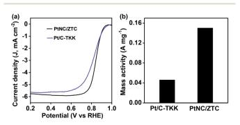
Fig. 4 (a) RDE ORR polarization curves at 1600 rpm and (b) mass activity at 0.8 V of PtNC/ZTC and Pt/C-TKK in 0.1 M HClO $_4$ .
