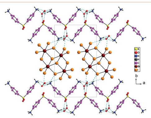
Fig. 3 Projection along the c axis of the cell content of  $(H_2DDS)[Bi_4|_{16}]$ . The dotted lines indicate hydrogen bonds.
