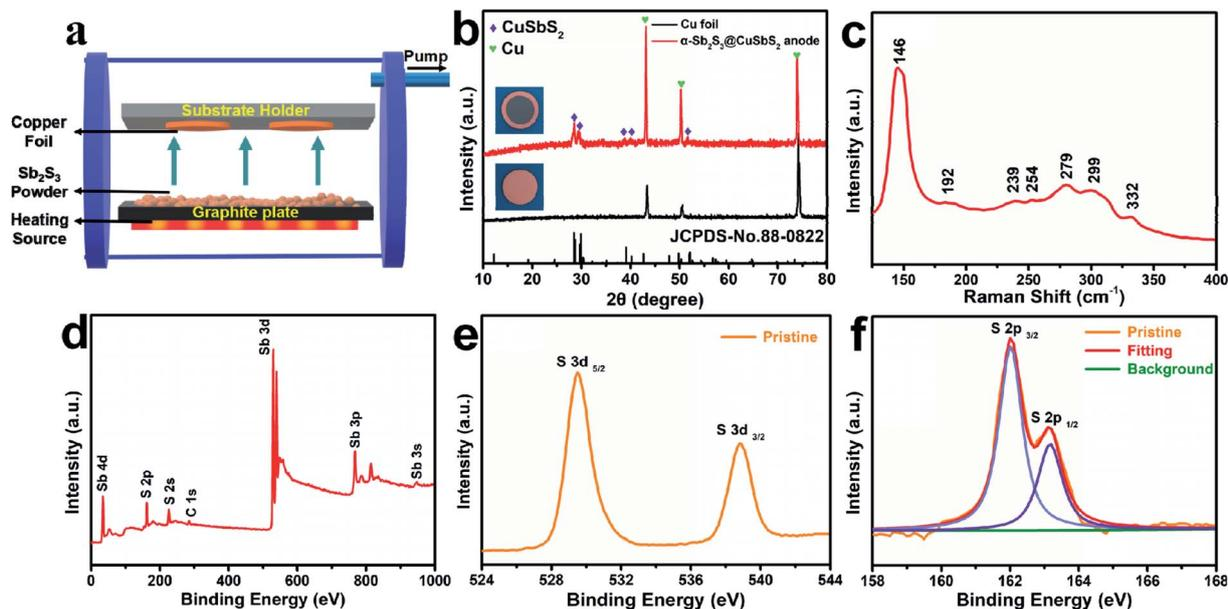
Fig. 1 (a) Schematic diagram of the synthesis of electrode by CSS device. (b) XRD patterns of pure copper foil and as-prepared electrode. (c) Raman spectra of the  $\alpha$ - $\text{Sb}_2\text{S}_3$ @ $\text{CuSbS}_2$  electrode. (d) XPS spectra typical survey spectrum of the  $\alpha$ - $\text{Sb}_2\text{S}_3$ @ $\text{CuSbS}_2$  electrode. (e) Sb 3d, (f) S 2p narrow scan spectra of the  $\alpha$ - $\text{Sb}_2\text{S}_3$ @ $\text{CuSbS}_2$  electrode.
