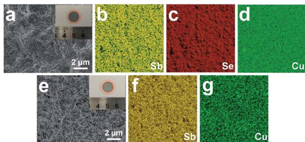
Fig. 7 Image of the electrode prepared by CSS process using  $\text{Sb}_2\text{Se}_3$  and Sb as raw material. The SEM of (a) the  $\text{Sb}_2\text{Se}_3$ -electrode and (e) the Sb-electrode. Individual elemental maps corresponding to the respective constituent elements for (b, c, and d) the  $\text{Sb}_2\text{Se}_3$ -electrode and (f and g) the Sb-electrode.
