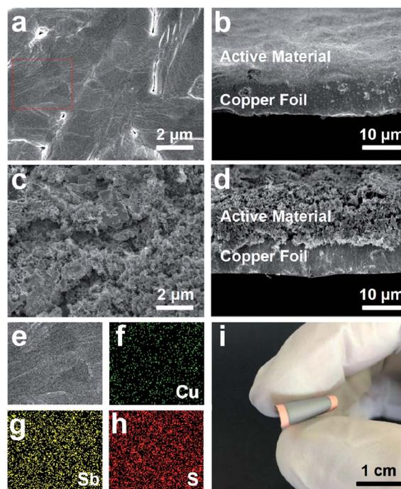
Fig. 2 (a) and (b) Surface and cross-section SEM images of  $\alpha$ - $\text{Sb}_2\text{S}_3$ @ $\text{CuSbS}_2$  electrode. (c) and (d) Surface and cross-section SEM images of traditional electrode. (e) EDS mapping of  $\alpha$ - $\text{Sb}_2\text{S}_3$ @ $\text{CuSbS}_2$  electrode (red area in (a)). (f) Cu (green). (g) Sb (yellow). (h) S (red). (i) Image of curved electrode.
