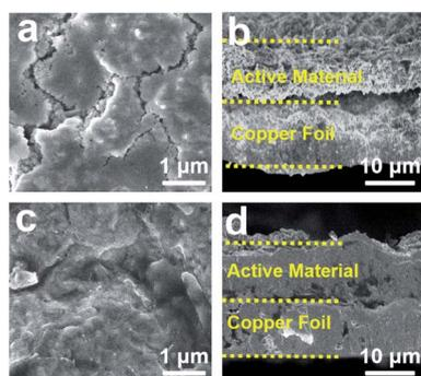
Fig. 6 (a) and (b) The traditional electrode SEM images of the electrode surface and cross-section after 30 cycles at a current density of  $0.1 \text{ A g}^{-1}$ . (c) and (d) The  $\alpha$ - $\text{Sb}_2\text{S}_3$ @ $\text{CuSbS}_2$  electrode SEM images of the electrode surface and cross-section after 30 cycles at a current density of  $0.1 \text{ A g}^{-1}$ .
